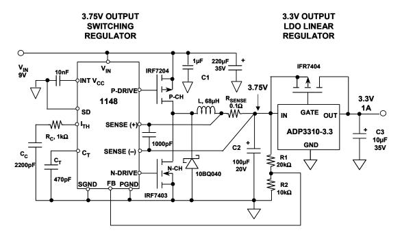
Figure 9.62: A Linear Post-Regulator Operating After a Switching/Linear Regulator is Capable of Low Noise, as Well as Good DC Efficiency
