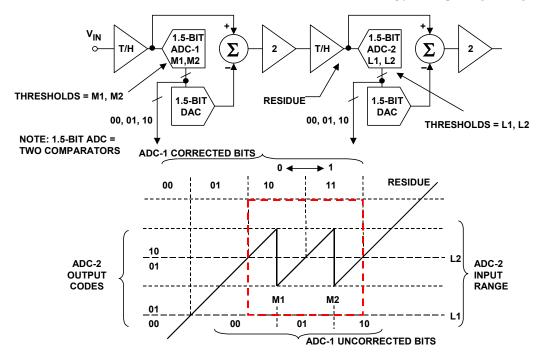
Figure 3.79: 1.5-Bit per Stage Pipeline Showing Error Corrected Range
