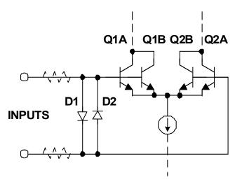
**Figure 9.83:** An Op Amp Input Stage With D1-D2 Input Differential Overvoltage Protection Network
