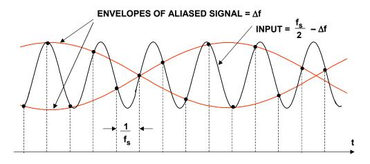
NOTE: INPUT IS SLIGHTLY LESS THAN f<sub>s</sub>/2
