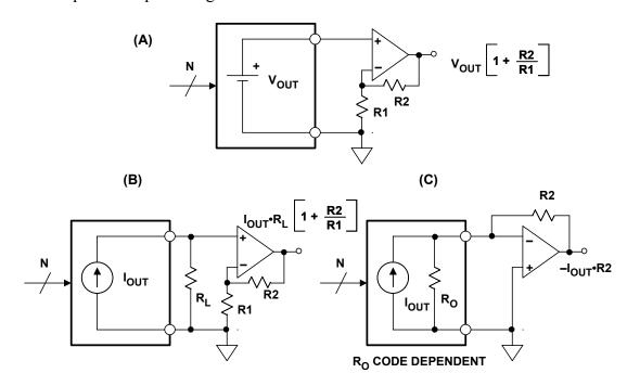
Figure 6.67: Buffering DAC Outputs with Op Amps
