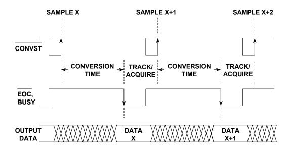
Figure 3.57: Typical SAR ADC Timing
