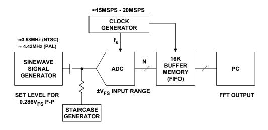
Figure 5.87: Digital Differential Gain and Phase Measurements
