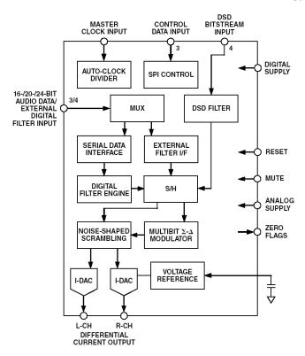
**Figure 8.68:** AD1955 High Performance Multibit  $\Sigma$ - $\Delta$  DAC
