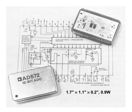
Figure 4.8: AD572 12-Bit, 25-µs ADC, 1977
