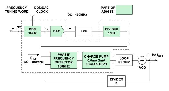
Figure 8.171: DDS Single Loop Upconversion Using the AD9858
