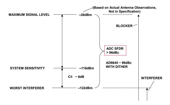
Figure 8.120: AMPS Spurious Requirements
