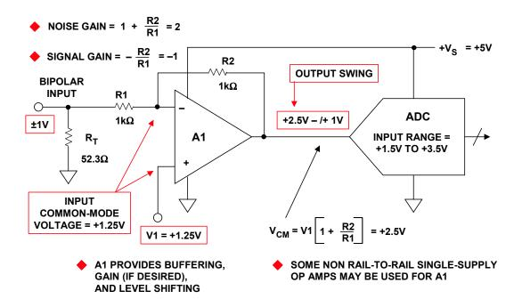
Figure 6.11: Single-Ended Single-Supply DC-Coupled Level Shifter
