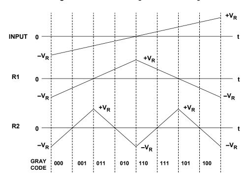
Figure 3.95: Input and Residue Waveforms for 3-Bit Folding ADC
