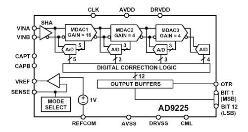
Figure 3.85: AD9225 12-Bit 25-MSPS CMOS ADC, 1998
