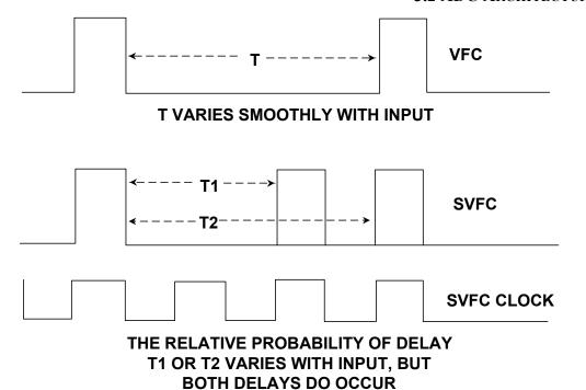
Figure 3.111: VFC and SVFC Waveforms
