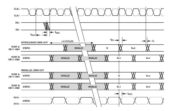
Figure 6.58: AD9430 Demuxed CMOS Output Data Timing
