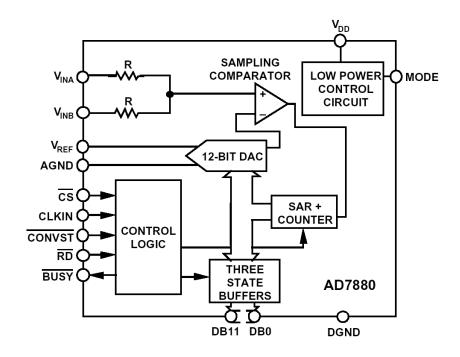
**Figure 1.51:** AD7880 12-Bit, 66-kSPS, Single +5 V, LC<sup>2</sup>MOS Sampling SAR ADC, 1990
