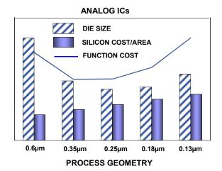
Figure 4.16: Fab Process Geometry Has a Different Effect on Analog Cost
