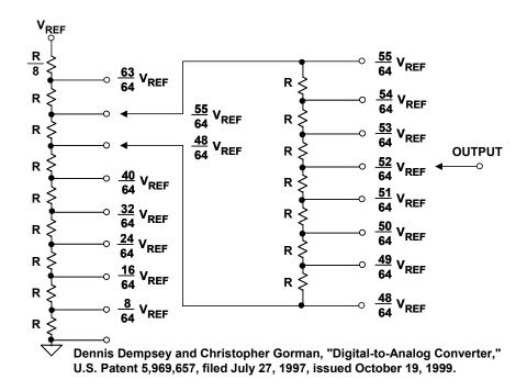
Figure 3.25: Segmented Unbuffered String DACs Use Patented Architecture
