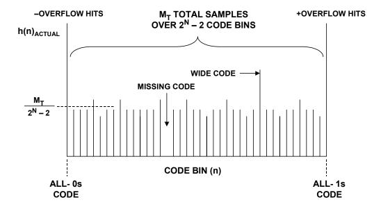
Figure 5.39: Histogram for Linear Ramp Test
