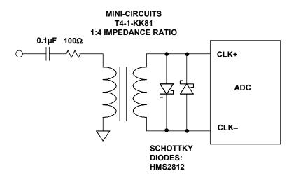
Figure 6.95: Single-Ended to Differential Conversion Using RF Transformer
