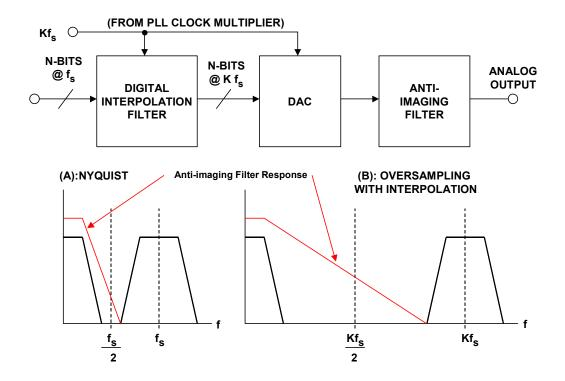
Figure 3.30: Oversampling Interpolating DAC
