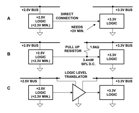
Figure 9.164: +2.5-V to +3.3-V Interface Analyzed
