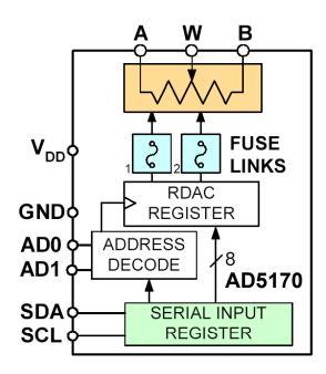
**Figure 8.59:** AD5170 256-Position Two-Time Programmable I<sup>2</sup>C Digital Potentiometer
