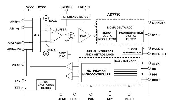
Figure 3.141: AD7730 Sigma-Delta Single-Supply Bridge ADC
