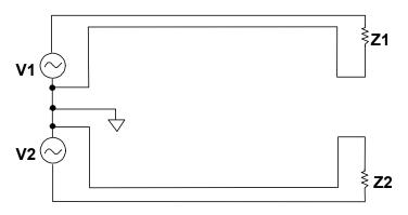
Figure 9.12: Proper Signal Routing and Layout can Reduce Inductive Coupling
