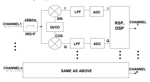
Figure 8.111: Digital Receiver Using Baseband Sampling and Digital Processing
