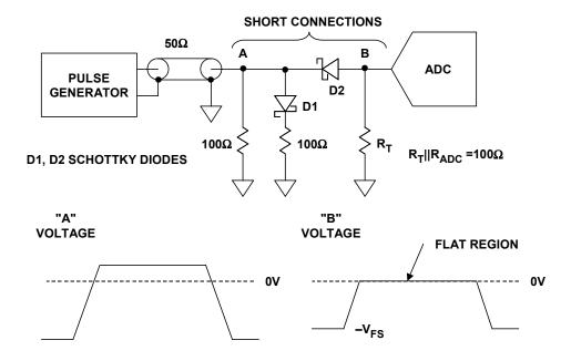
Figure 5.81: A Simple Flat Pulse Generator
