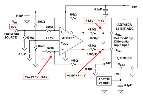
Figure 6.36: AD8137 Driving AD7450A 12-Bit, 1-MSPS, 3-V ADC
