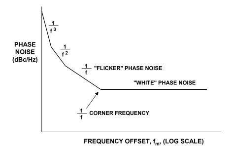
Figure 6.83: Oscillator Phase Noise in dBc/Hz vs. Frequency Offset
