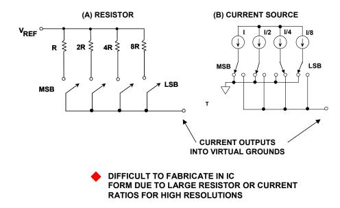
Figure 3.13: Current-Mode Binary-Weighted DACs
