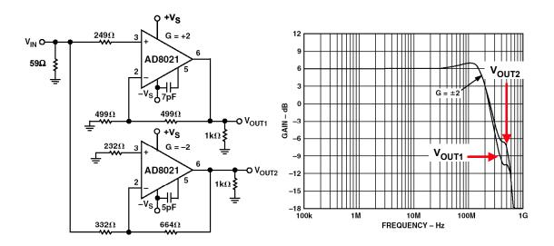
**Figure 6.46:** Balanced AD8021 Driver Compensated to Give Matched Gains to > 100 MHz
