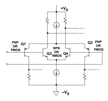
Figure 6.7: A True Rail-to-Rail Input Stage
