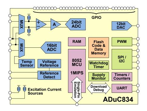
**Figure 8.183:** Standard Σ-Δ MicroConverter® Products: ADuC816/ADuC824/ADuC836/ADuC834
