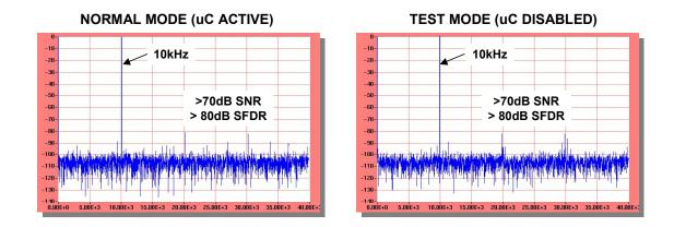
Figure 8.181: MicroConverter SAR ADC Performance
