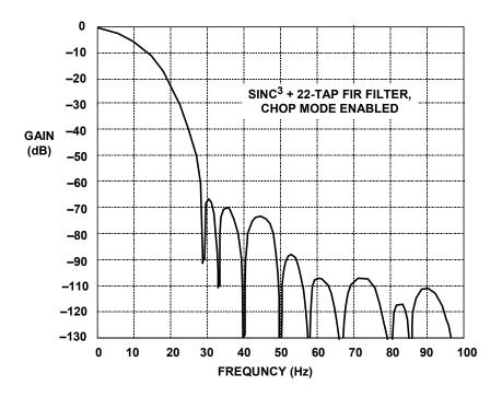
Figure 3.142: AD7730 Digital Filter Response
