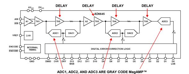
**Figure 3.88:** AD6645 14-Bit, 105-MSPS ADC, 2003 (80-MSPS Version Released in 2002)
