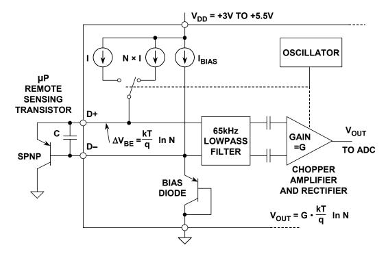
**Figure 8.25**: ADM1023 Microprocessor Temperature Monitor Input Conditioning Circuits
