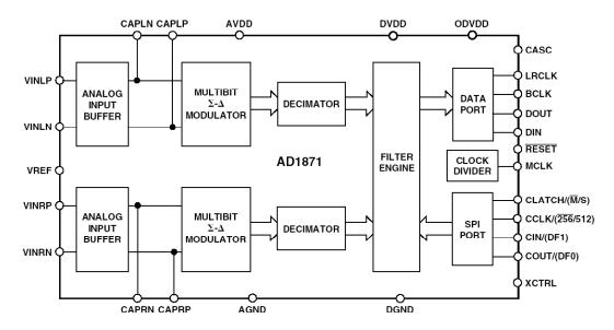
**Figure 8.67:** AD1871 Stereo Audio, 24-Bit, 96-kSPS Multibit  $\Sigma$ - $\Delta$  ADC
