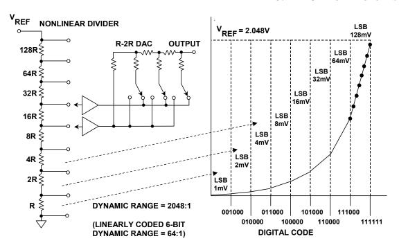
Figure 3.33: Nonlinear 6-Bit Segmented DAC
