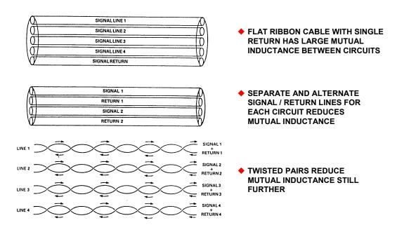
Figure 9.13: Mutual Inductance and Coupling Within Signal Cabling
