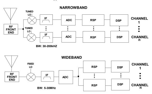
Figure 8.115: Narrowband Versus Wideband Digital Receiver
