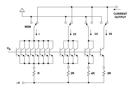
Figure 1.21: "Quad Switch" DAC Building Block with External
