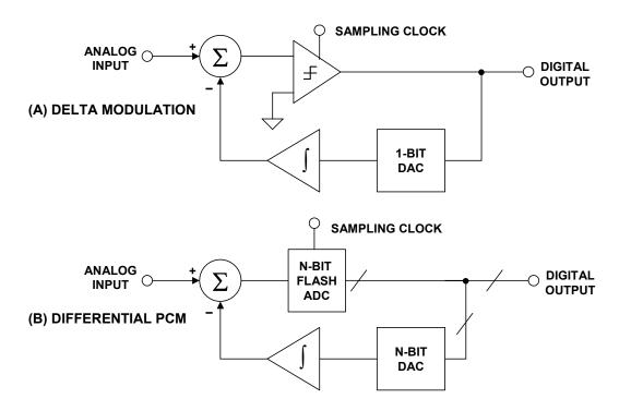
Figure 3.119: Delta Modulation and Differential PCM
