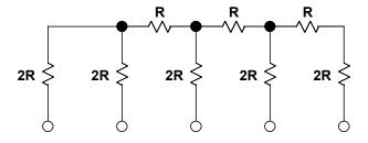
Figure 3.15: 4-Bit R-2R Ladder Network
