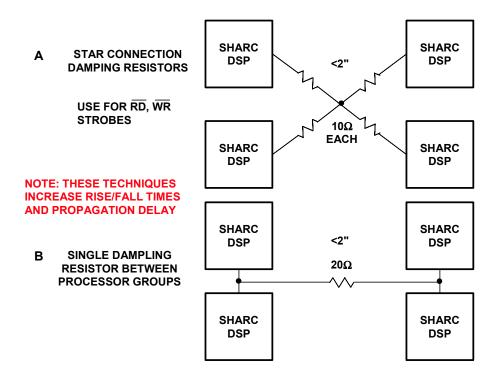
Figure 9.146: Series Damping Resistors for High Speed DSP Interconnections
