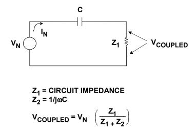
Figure 9.48: Capacitive Coupling Equivalent Circuit Model
