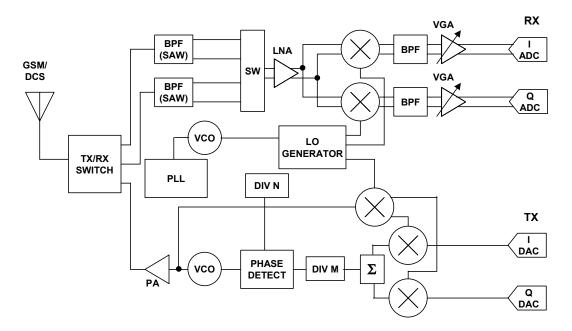
**Figure 8.149:** Superhomodyne™ Direct Conversion Dual-Band Transceiver Using Othello
