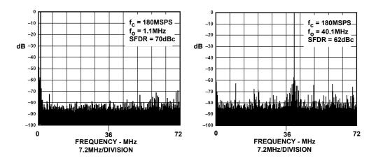
Figure 5.21: AD9851 10-Bit, 180-MSPS DDS Spectral Output
