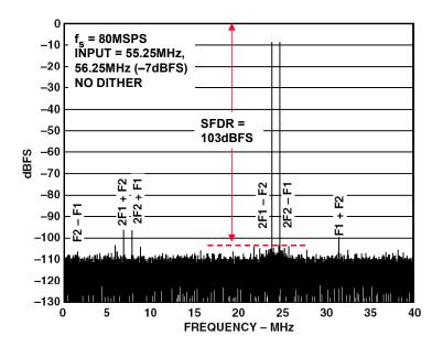
Figure 8.125: AD6645 Two-Tone Intermodulation Performance
