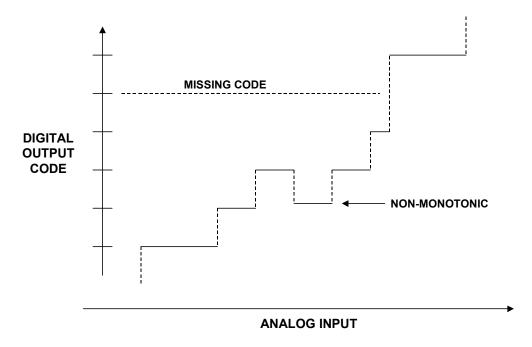
Figure 2.22: Non-Monotonic ADC with Missing Code
