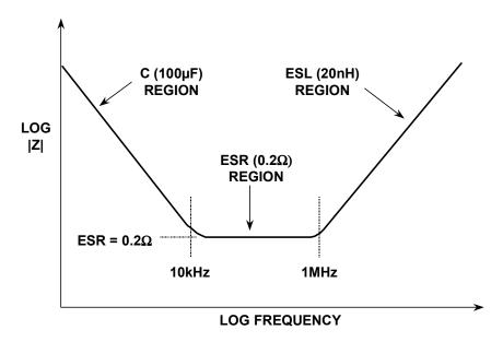
Figure 9.69: Electrolytic Capacitor Impedance Versus Frequency
