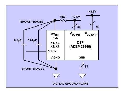
Figure 9.32: Grounding DSPs with Internal Phase-Locked-Loops (PLLs)
