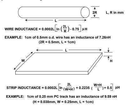
Figure 9.9: Wire and Strip Inductance Calculations
