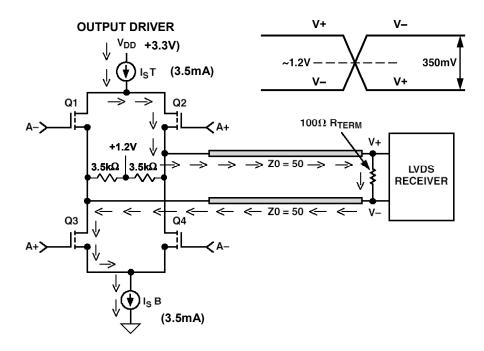
Figure 6.52: LVDS Driver Designed in CMOS
