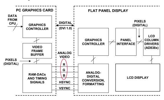
Figure 8.94: Flat Panel Analog and Digital Interfaces
