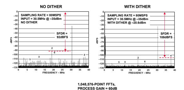
Figure 8.135: AD6645 Undithered and Dithered SFDR FFT Plot
