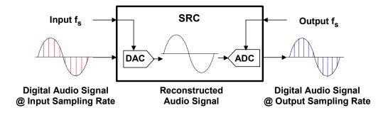
Figure 8.75: The Concept of a Sample Rate Converter
