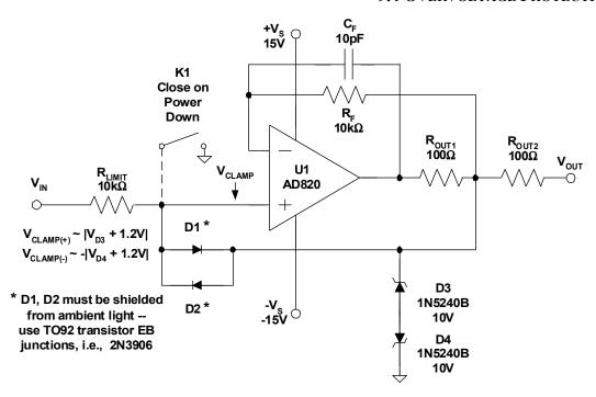
Figure 9.77: Bootstrapping the D1-D2 Protection Network Reduces Diode Leakage to Negligible Levels, and is Voltage-Programmable for Clamp Level
