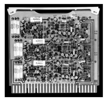
Figure 4.6: Double-Sided PC Board from HS-810 ADC
