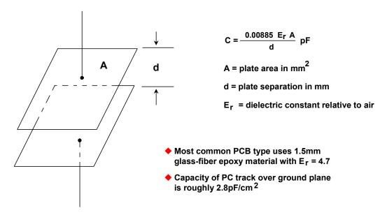
Figure 9.47: Capacitance of Two Parallel Plates
