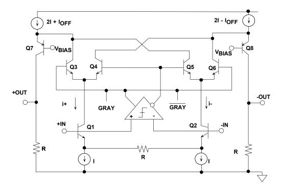
Figure 3.99: A Modern Current-Steering MagAMP™ Stage
