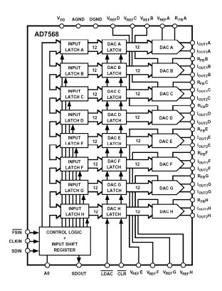
Figure 1.47: AD7568 Octal 12-Bit LC<sup>2</sup>MOS MDAC, 1991
