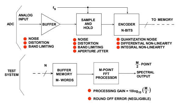
Figure 2.45: ADC Model Showing Noise and Distortion Sources
