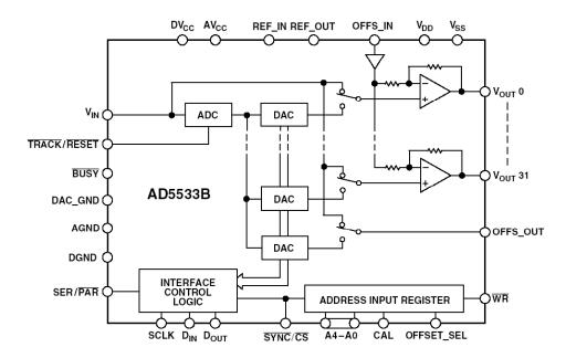
Figure 8.51: AD5533B 32-Channel Precision Infinite Sample-and-Hold
