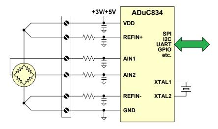
Figure 8.188: Bridge Transducer Interfacing Using a MicroConverter
