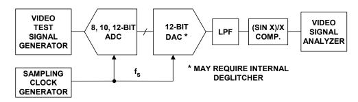
Figure 5.83: Composite Video Test Setup Using Analog Methods
