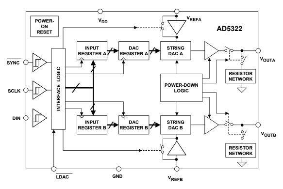
Figure 6.62: AD5322 12-BIT, 100-kSPS Dual Serial DAC
