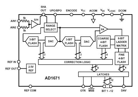
Figure 1.52: AD1671 12-Bit, 1.25-MSPS Sampling BiCMOS ADC, 1992
