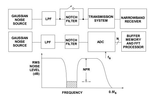
Figure 2.63: Noise Power Ratio (NPR) Measurements
