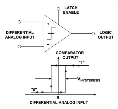
Figure 3.45: The Comparator: A 1-Bit ADC
