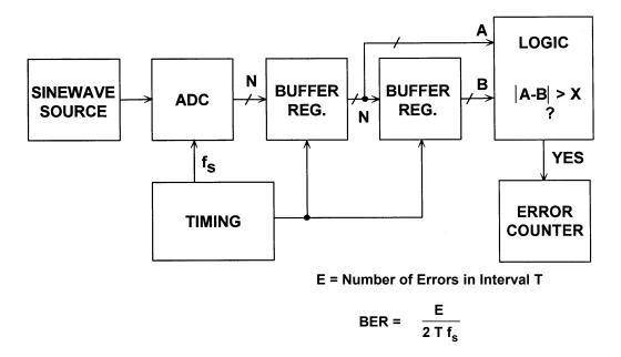
Figure 2.89: ADC Bit Error Rate Test Setup
