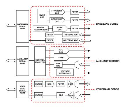
Figure 8.147: AD6521 Baseband/Voiceband Codec Simplified Block Diagram
