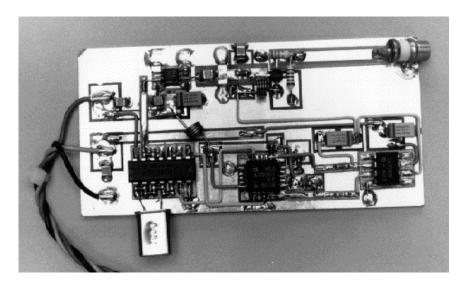
Figure 9.176: A "Solder-Mount" Constructed Prototype Board
