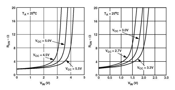
Figure 9.160: ON Resistance vs. Input Voltage for ADG3257 Bus Switch
