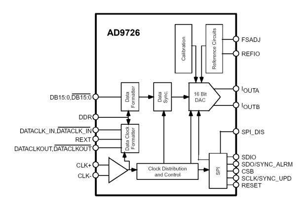
Figure 6.66: AD9726 16-Bit, 600+ MSPS DAC with LVDS Inputs
