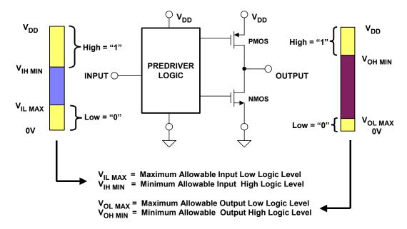
Figure 9.156: Typical CMOS IC Output Driver Configuration
