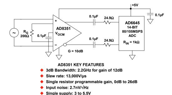
Adjustable output common-mode voltage
