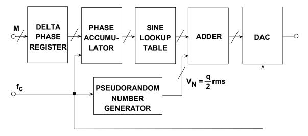
**Figure 8.165:** Injection of Digital Dither in a DDS System to Randomize Quantization Noise and Increase SFDR
