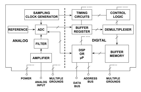
Figure 9.34: Analog and Digital Circuits Should be Partitioned on PCB Layout
