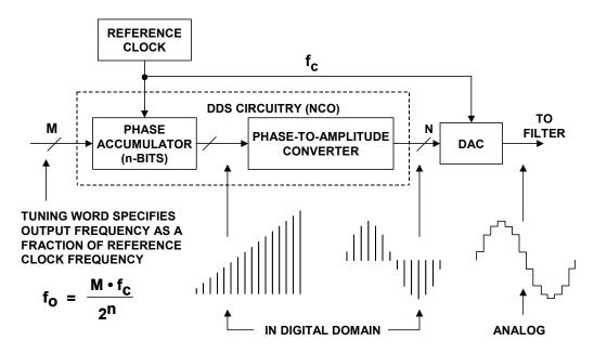
Figure 8.162: Signal Flow Through the DDS Architecture
