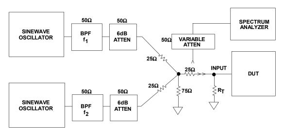
Figure 5.71: Low Distortion Two-Tone Generator
