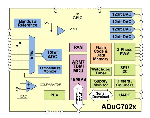
Figure 8.194: ADuC702x ARM7-Based MicroConverter Products
