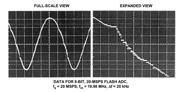
Figure 5.48: Beat Frequency and Envelope Tests Show ADC AC Nonlinearities
