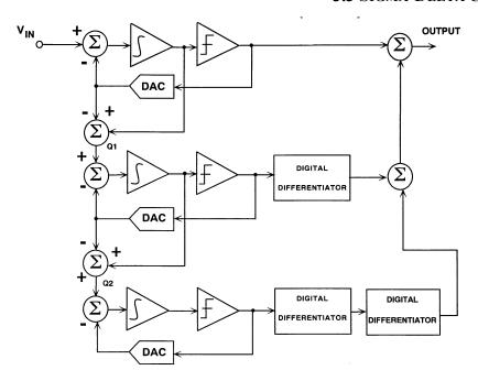
Figure 3.140: Multi-Stage Noise Shaping Sigma-Delta ADC (MASH)
