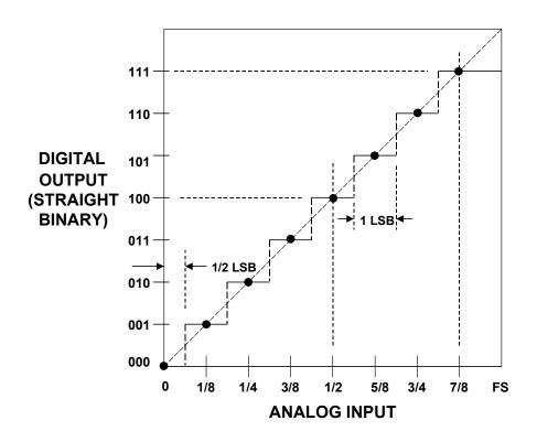
Figure 2.5: Transfer Function for Ideal Unipolar 3-bit ADC
