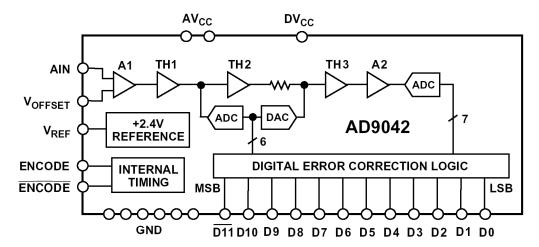
Figure 1.54: AD9042 12-Bit 41-MSPS XFCB, Sampling ADC, 1995
