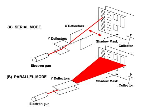
Figure 1.11: The Electron Beam Coder
