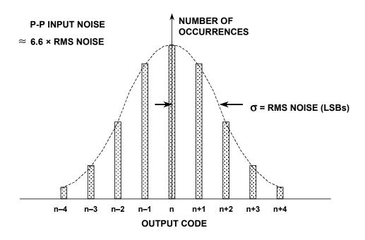
Figure 5.43: Measuring Input-Referred Noise Using "Grounded Input" Histogram
