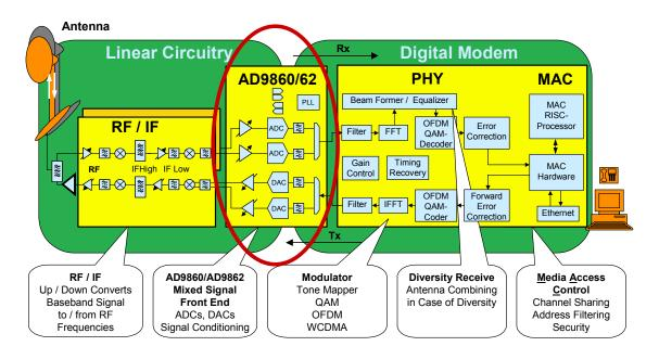
Figure 4.21: AD9860/AD9862: Broadband Wireless OFDM Modem
