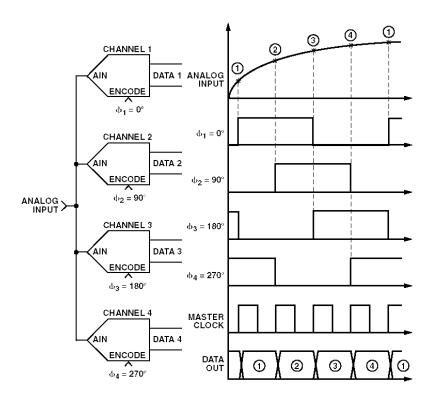
Figure 8.150: Time-Interleaved ADCs
