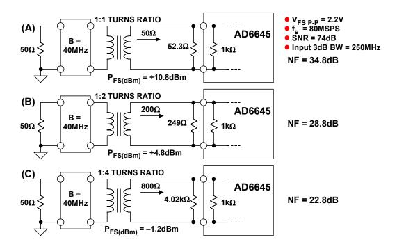
Figure 2.73: Using RF Transformers to Improve Overall ADC Noise Figure
