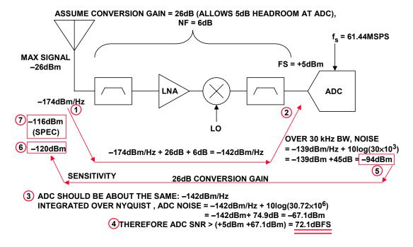
Figure 8.121: AMPS Receiver Sensitivity Requirements
