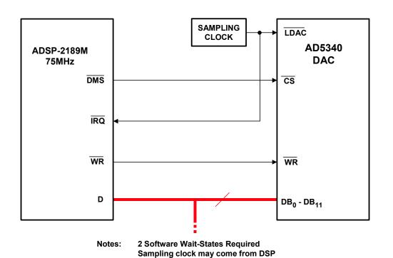
Figure 6.65: AD5340 DAC Parallel Interface to ADSP-2189M
