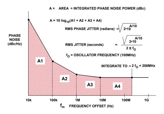
Figure 6.84: Calculating Jitter from Phase Noise
