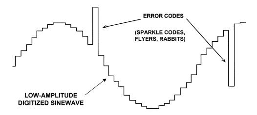
Figure 2.87: Exaggerated Output of ADC Showing Error Codes
