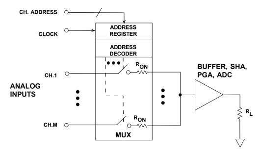
Figure 8.33: Simplified Diagram of a Typical Analog Multiplexer
