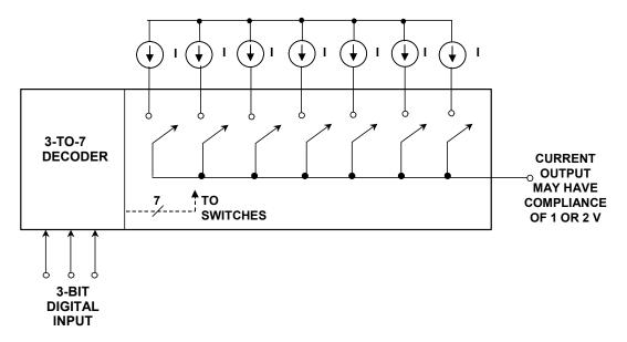
Figure 3.8: Current Sources Improve the Basic Current-Output Thermometer DAC
