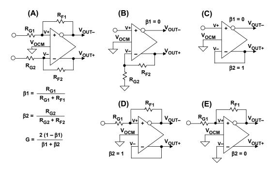
Figure 6.34: Some Configurations for Differential Amplifiers
