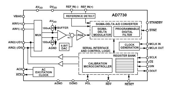
Figure 1.55: AD7730 24-Bit Signal-Conditioning  $\Sigma$ -Δ ADC, 1997
