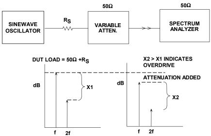
Figure 5.72: Verifying Spectrum Analyzer Sensitivity to Input Overdrive
