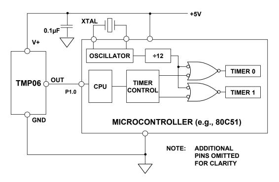
Figure 8.22: Interfacing TMP06 to a Microcontroller
