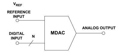
ANALOG OUPTUT =  $V_{REF} \times DIGITAL INPUT \times CONSTANT$
