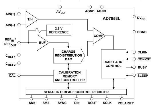
Figure 6.53: AD7853/AD7853L +3-V Single-Supply 12-Bit 200-/100-kSPS Serial Output ADC
