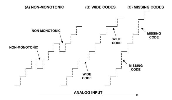
Figure 2.23: Errors Associated with Improperly Trimmed Subranging ADC
