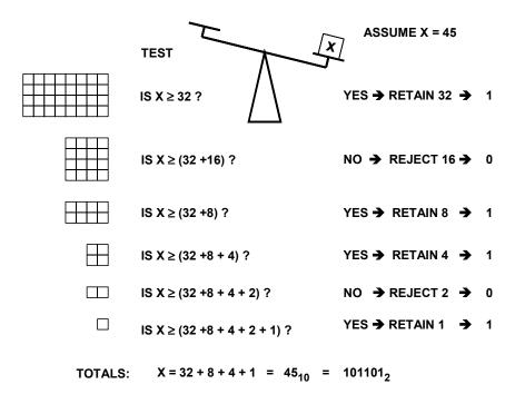
Figure 1.22: Successive Approximation ADC Algorithm
