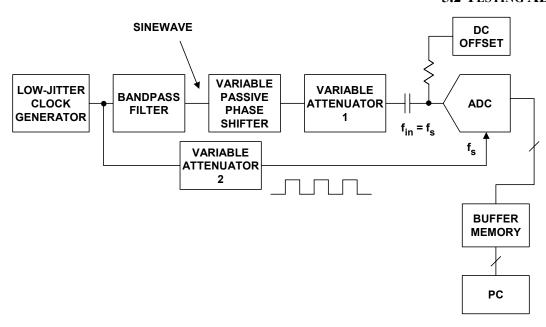
Figure 5.76: Locked-Histogram Test Setup for Measuring ADC Aperture Jitter
