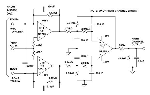
**Figure 6.75:** A 75-kHz 4-Pole Gaussian Active Filter for Buffering the Output of the AD1853 Stereo DAC
