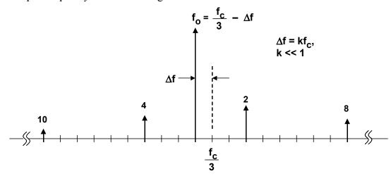
**Figure 5.23:** Location of Even Harmonics for  $f_0 = f_c/3 - \Delta f$
