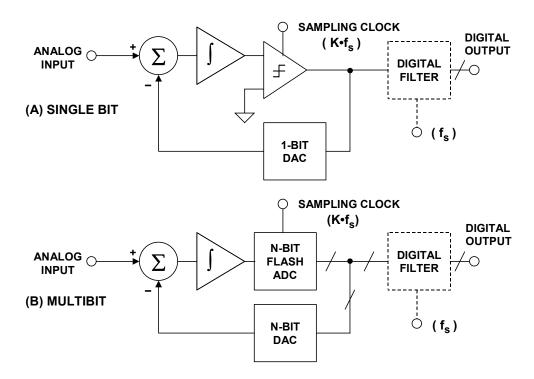
Figure 3.121: Single and Multibit Sigma-Delta ADCs
