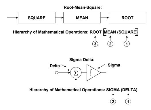
**Figure 3.123:** Sigma-Delta ( $\Sigma$ -Δ) or Delta-Sigma ( $\Delta$ - $\Sigma$ )?
