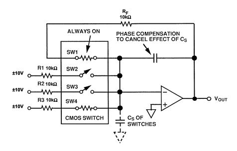
Figure 7.78: Applying the Analog Switch: Using "Dummy" Switch in Feedback to Minimize Gain Error Due to △R<sub>ON</sub>
