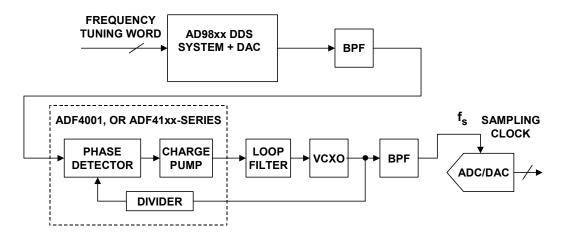
Figure 6.93: A Simple "Hybrid" Sampling Clock Generator
