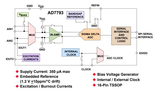
Figure 8.18: AD7793 24-bit Σ-Δ ADC
