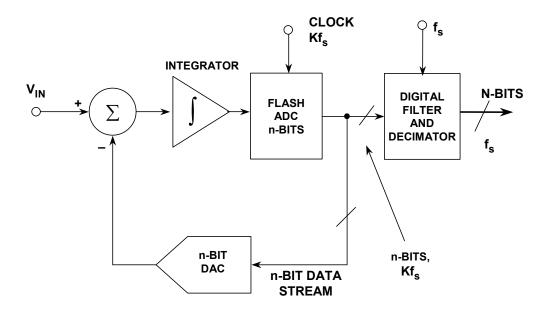
Figure 3.135: Multi-Bit Sigma-Delta ADC
