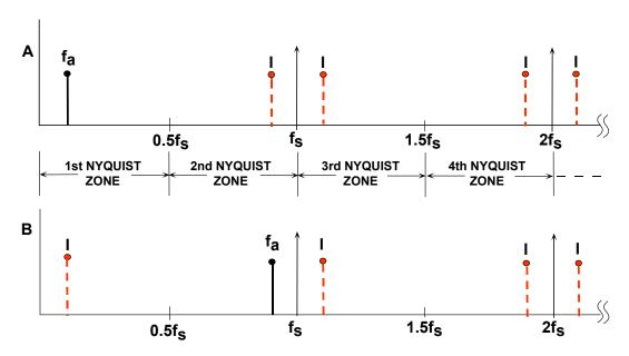
**Figure 2.31:** Analog Signal  $f_a$  Sampled @  $f_s$  Using Ideal Sampler Has Images (Aliases) at  $|\pm Kf_s \pm f_a|$ , K = 1, 2, 3, ...
