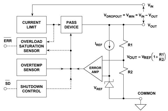
Figure 9.54: Block Diagram of a Voltage Regulator
