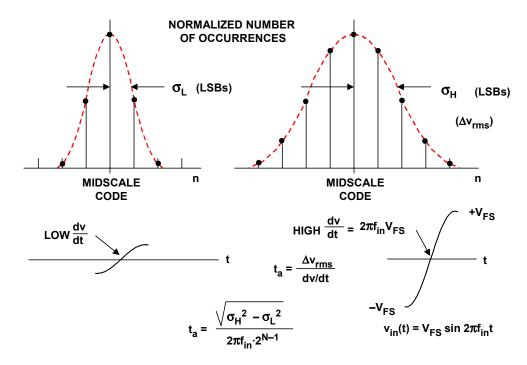
Figure 5.77: Calculating Aperture Jitter Based on Locked-Histogram Test
