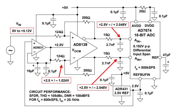
Figure 6.47: AD8139 Low Noise Differential Driver in a 18-bit ADC Application
