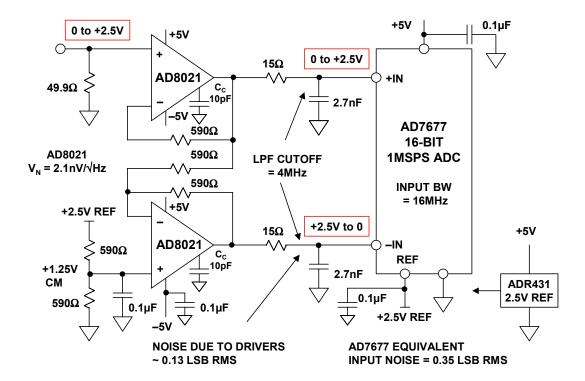
Figure 6.45: A True 16-bit ADC Requires a True 16-Bit Driver
