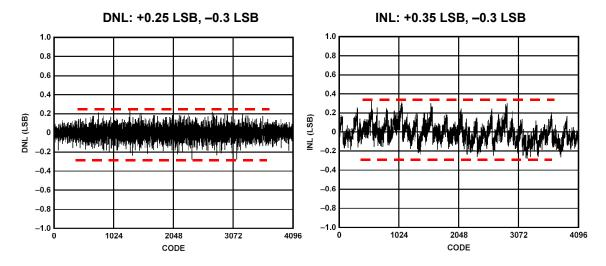
Figure 5.42: Typical Static DNL and INL Histogram Plots for AD9236 12-Bit, 80-MSPS ADC
