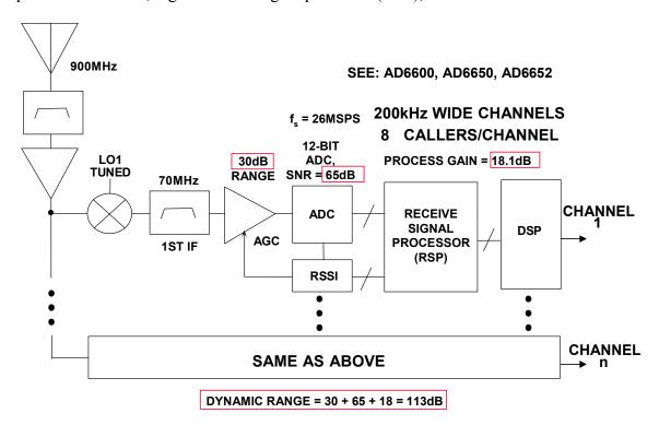
Figure 8.112: Narrowband IF Sampling GSM/EDGE Digital Receiver
