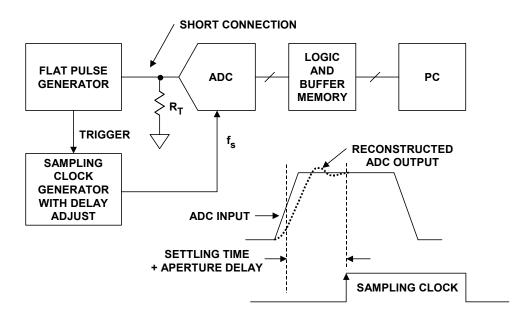
Figure 5.80: Settling Time Test Setup
