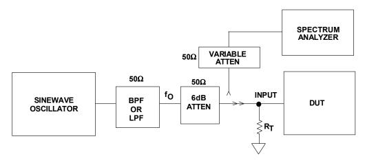
Figure 5.70: Low Distortion Single-Tone Generator
