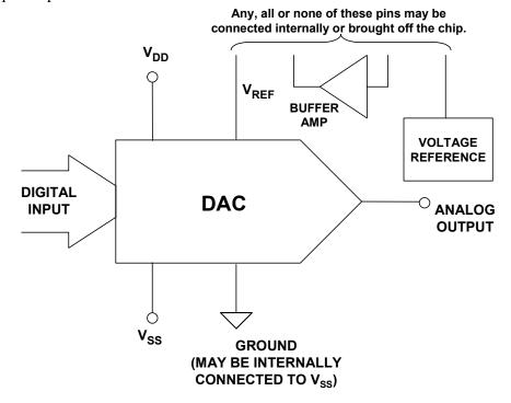
Figure 3.2: DAC with Reference and Buffer
