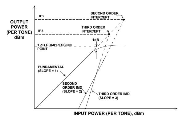
**Figure 2.58:** Definition of Intercept Points and 1-dB Compression Points for Amplifiers
