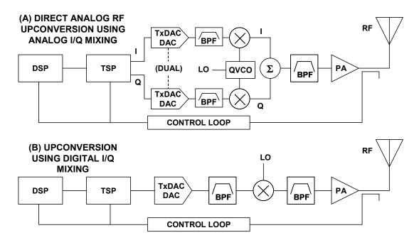
Figure 8.139: Simplified Wireless Transmitter Architectures
