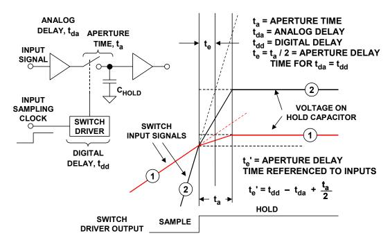
Figure 2.77: Sample-and-Hold Waveforms and Definitions
