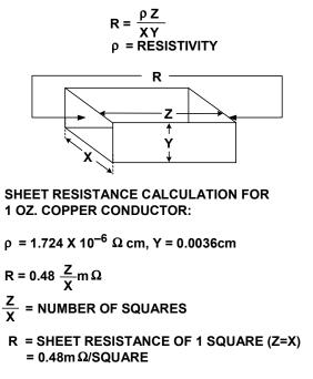
**Figure 9.16:** Calculation of Sheet Resistance and Linear Resistance for Standard Copper PCB Conductors
