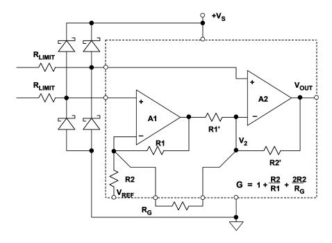
Figure 9.87: Single-Supply In-Amps May or May Not Require External Protection in the Form of Resistors and Clamp Diodes—
