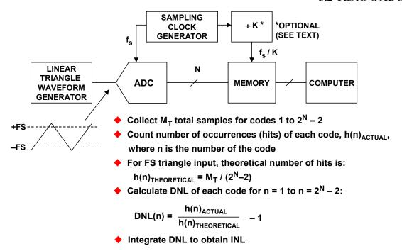
Figure 5.38: Histogram (Code Density) Test Setup
