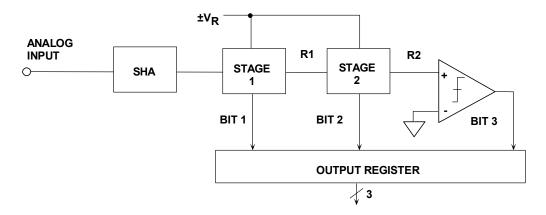
Figure 3.91: 3-bit Serial ADC with Binary Output
