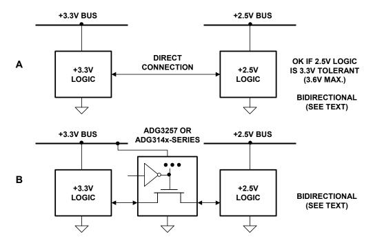
Figure 9.163: +3.3-V to +2.5-V Interface
