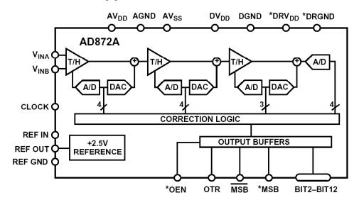
Figure 1.53: AD872 12-Bit 10-MSPS BiCMOS Sampling ADC, 1992
