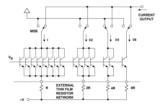
Figure 3.20: Binary-Weighted 4-Bit DAC, the AD550 "µDAC" Quad Switch
