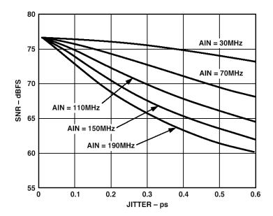
Figure 2.82: AD6645 SNR Versus Jitter
