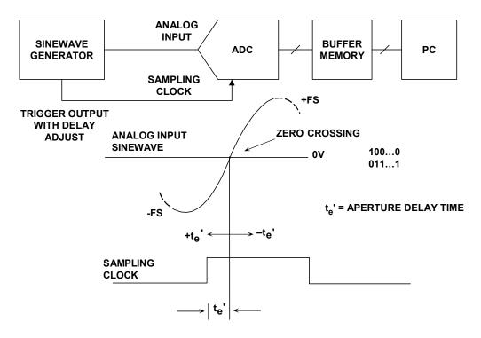
Figure 5.78: Measuring Aperture Delay Time
