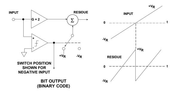
Figure 3.90: Single-Stage Transfer Function for Binary ADC
