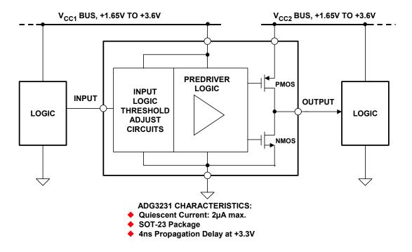
Figure 9.166: ADG3231 Low Voltage Logic Level Translator
