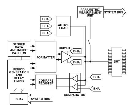
Figure 8.52: Infinite Sample-and-Holds (ISHAs)
