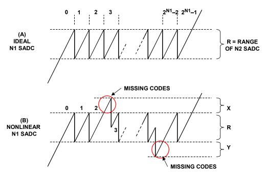
Figure 3.66: Residue Waveforms at Input of N2 Sub-ADC
