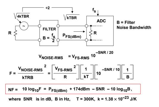
Figure 2.70: ADC Noise Figure in Terms of SNR, Sampling Rate, and Input Power
