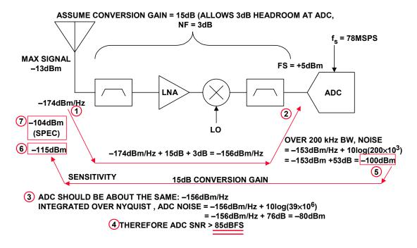
Figure 8.123: GSM 900 MHz Sensitivity Requirements (ADC SNR)
