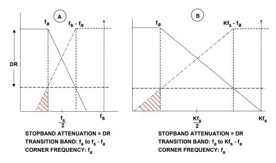
Figure 2.32: Oversampling Relaxes Requirements on Baseband Antialiasing Filter
