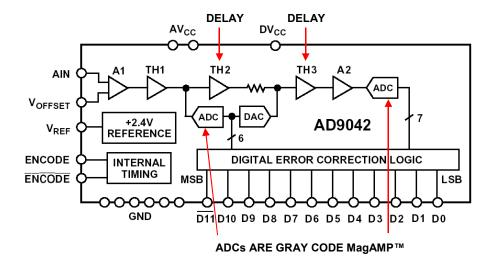
Figure 3.84: AD9042 12-Bit 41-MSPS ADC, 1995
