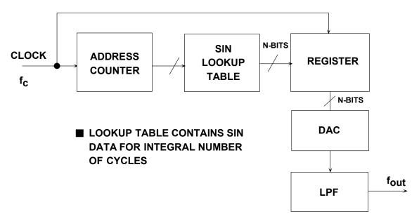
Figure 8.159: Fundamental Direct Digital Synthesis System
