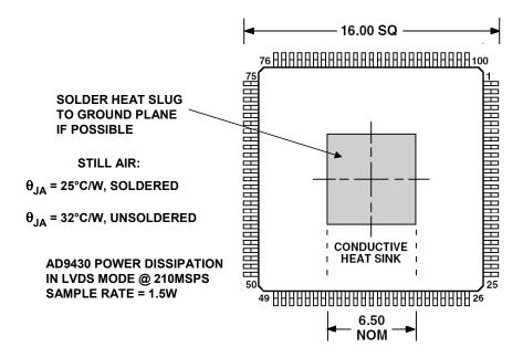
Figure 9.119: AD9430 100-Lead e-PAD TQFP
