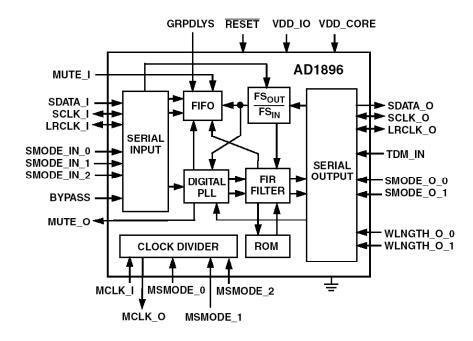
Figure 8.77: AD1896 192-kHz Stereo Asynchronous Sample Rate Converter
