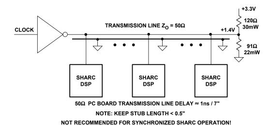
Figure 9.148: Clock Distribution Using End-of-Line Termination
