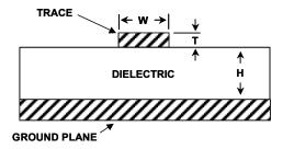
Figure 9.141: A Microstrip Transmission Line With Defined Impedance is Formed by a PCB Trace of Appropriate Geometry,
