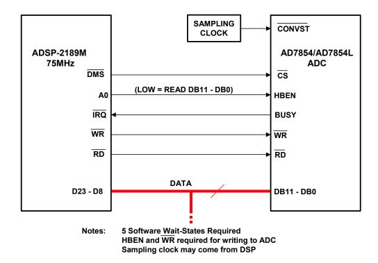
Figure 6.60: AD7854/AD7854L ADC Parallel Interface to ADSP-2189M
