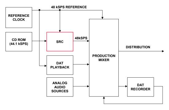
Figure 8.74: The Need for Sample Rate Converters (SRCs)
