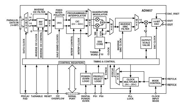
Figure 8.176: AD9857 200-MSPS, 14-Bit Quadrature Digital Upconverter
