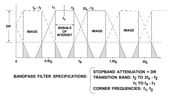
Figure 2.35: Antialiasing Filter for Undersampling
