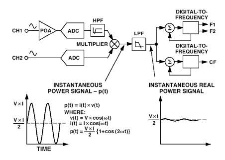
Figure 8.29: ADE7755 Energy Metering IC Signal Processing
