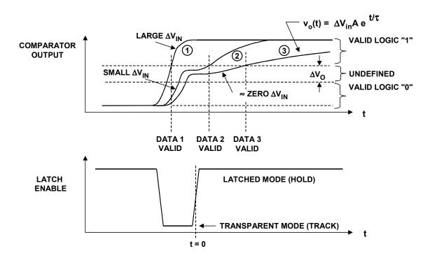
Figure 3.47: Comparator Metastable State Errors
