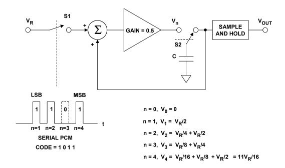
Figure 3.37: 4-Bit Cyclic Serial DAC
