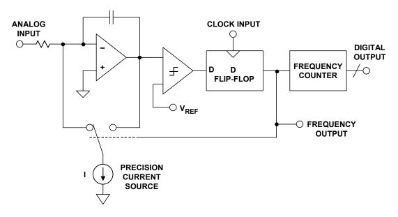
Figure 3.110: Synchronous VFC (SVFC)
