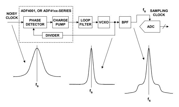
Figure 6.88: Using a Phase-Locked Loop (PLL) and Bandpass Filter to Condition a Noisy Clock Source
