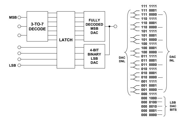
Figure 5.11: 3-Bit×4-Bit Segmented 7-Bit DAC Test Codes
