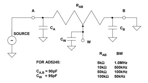
BW MEASURED FROM A TO W WITH B GROUNDED, MIDSCALE CODE, DRIVEN FROM A LOW IMPEDANCE SOURCE
