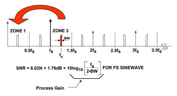
Figure 2.41: Undersampling and Oversampling Combined Results in Process Gain
