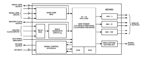
Figure 8.70: AD1953 SigmaDSP™ 3-Channel, 26-Bit Signal Processing DAC
