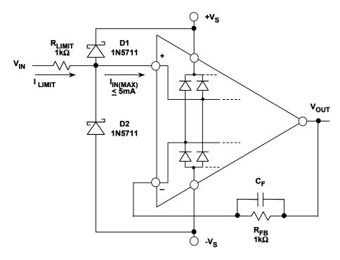
Figure 9.75: A General-Purpose Op Amp CM Overvoltage Protection Network Using Schottky Clamp Diodes with Current Limit Resistance
