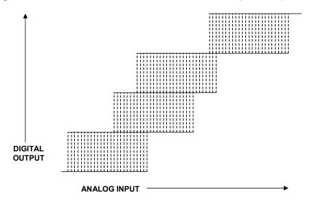
Figure 5.37: ADC Transfer Function With Relatively High Input-Referred Noise
