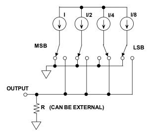
Figure 3.19: Binary-Weighted Current Sources Switched into a Load
