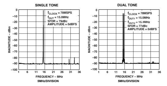
Figure 5.22: AD9744, 14-Bit, 165-MSPS TxDAC® Spectral Output
