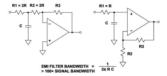
Figure 9.135: Simple EMI/RFI Noise Filters for Op Amp Circuits
