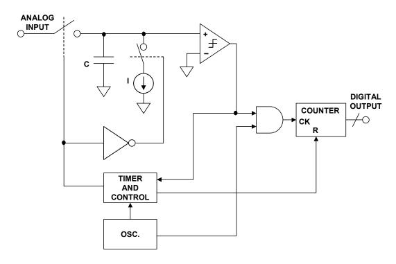
Figure 3.104: Charge Run-Down ADC
