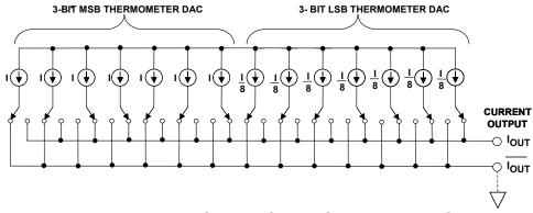
Figure 3.27: 6-Bit Current-Output Segmented DAC
