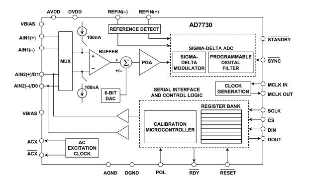
Figure 8.4: AD7730 Single-Supply Bridge ADC
