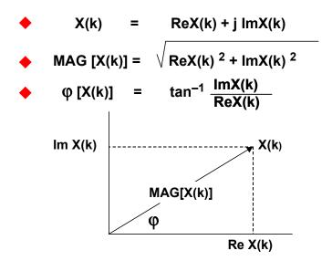
Figure 5.53: Converting Real and Imaginary DFT
