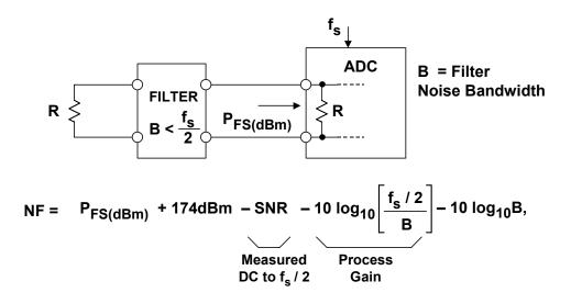
where SNR is in dB, B in Hz, T = 300K,  $k = 1.38 \times 10^{-23} \text{ J/K}$
