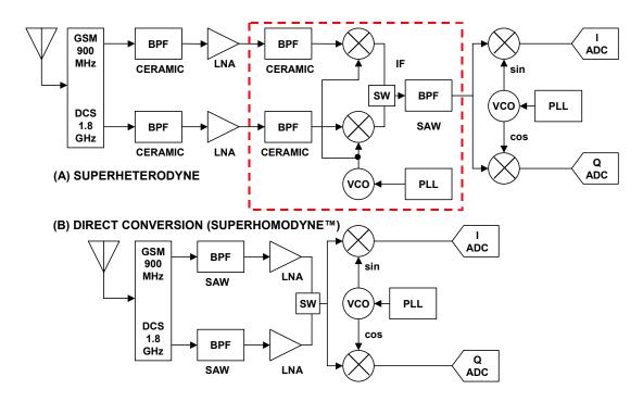
Figure 8.148: Direct Conversion Receiver Architecture Eliminates Components
