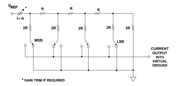
Figure 3.17: Current-Mode R-2R Ladder Network DAC
