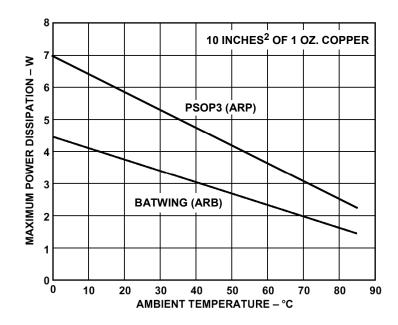
Figure 9.112: Thermal Characteristic Curves for the AD8016 BATWING (Lower) and PSOP3 (Upper) Packages, for T<sub>J(Max)</sub> Equal to 125 ℃
