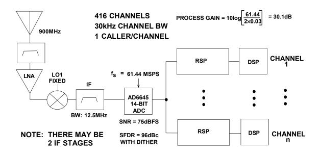
Figure 8.119: AMPS Wideband Digital Receiver
