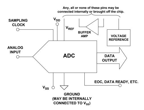
Figure 3.44: ADC with Reference and Buffer
