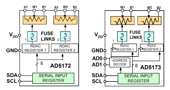
**Figure 8.58:** AD5172/AD5173 256-Position One-Time Programmable Dual-Channel I<sup>2</sup>C Digital Potentiometer
