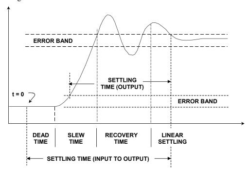
Figure 2.93: DAC Settling Time
