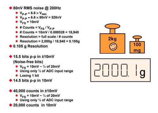
Figure 8.15: AD7730 Resolution @ 200-Hz Data Rate
