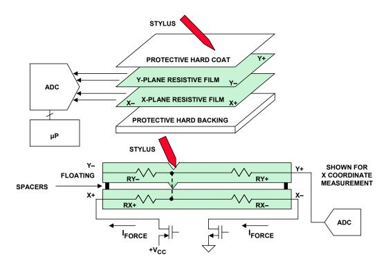
Figure 8.105: 4-Wire Resistive Touchscreen ADC Interface
