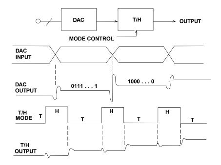
Figure 3.39: Deglitching DAC Outputs Using a Track-and-Hold
