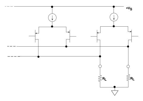
Figure 3.29: PMOS Transistor Current Switches
