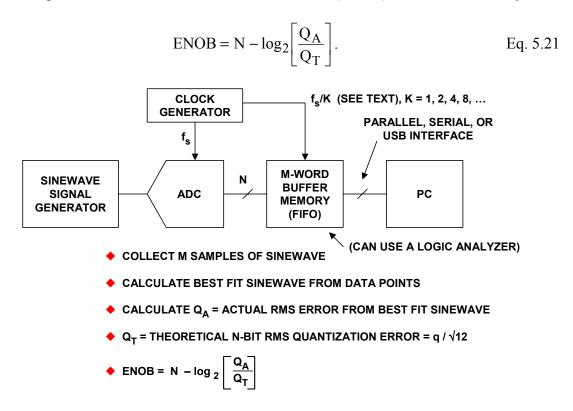
Figure 5.49: Sinewave Curve Fit Test Setup for Measuring ADC ENOB
