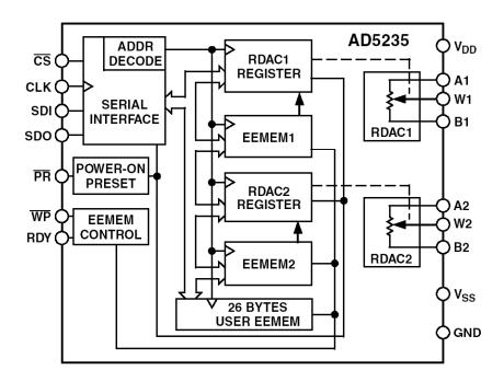
Figure 8.57: AD5235 Nonvolatile Memory, Dual 1024-Position Digital Potentiometers
