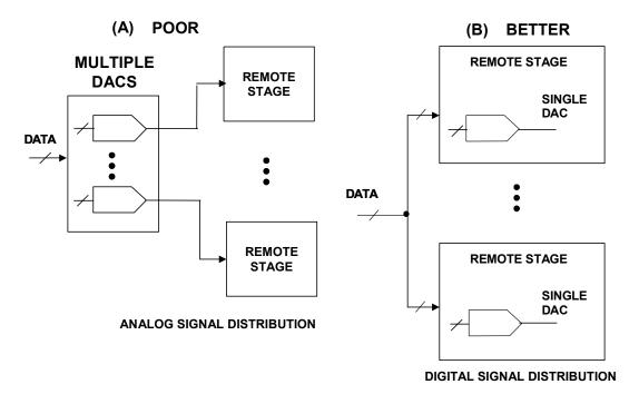
Figure 8.47: Remote, Multichannel Data Distribution
