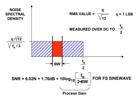
Figure 2.40: Quantization Noise Spectrum
