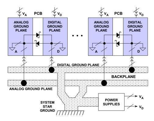
Figure 9.25: Separating Analog and Digital Ground Planes
