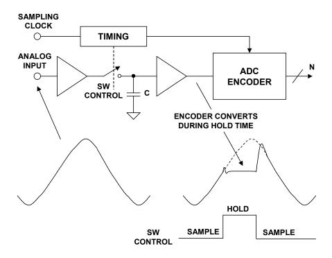
Figure 2.27: Sample-and-Hold Function Required for Digitizing AC Signals
