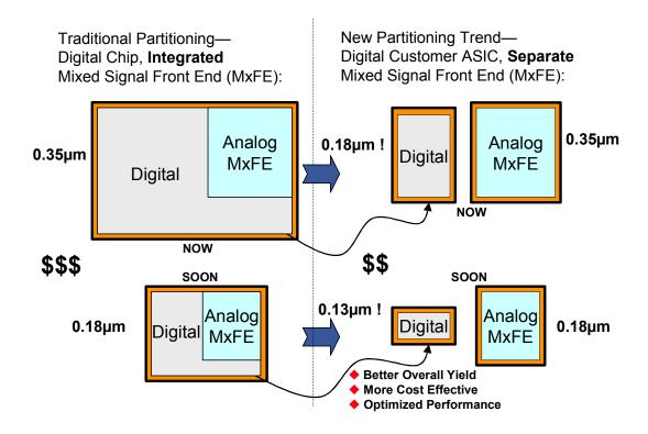
Figure 4.17: Smart Analog/Digital Partitioning
