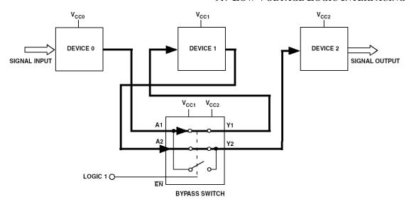
Figure 9.168: ADG3233 Bypass Switch in Normal Mode
