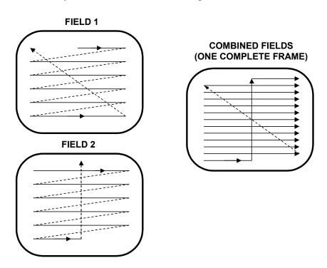
Figure 8.78: Standard Broadcast Television Interlace Format
