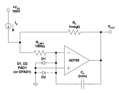
**Figure 9.80:** A Low Bias Current FET Input Op Amp I/V Converter With Overvoltage Protection Network R<sub>LIMIT</sub> and D1
