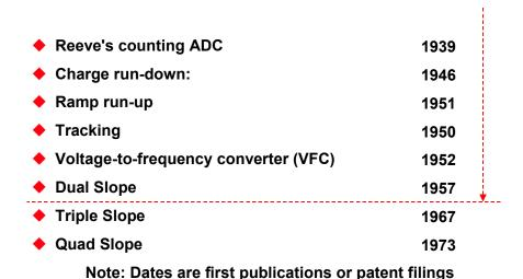
Figure 3.102: Counting and Integrating ADC Architecture Timeline
