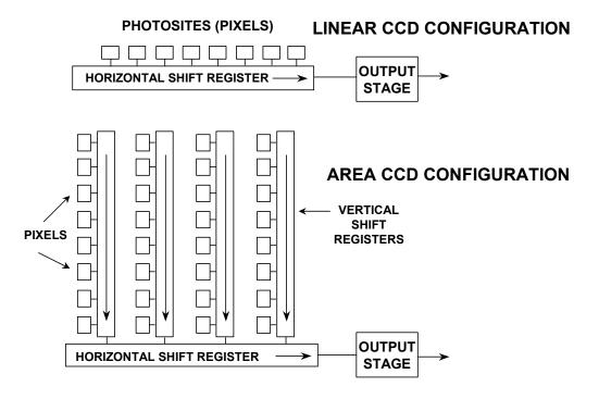
Figure 8.99: Linear and Area CCD Arrays
