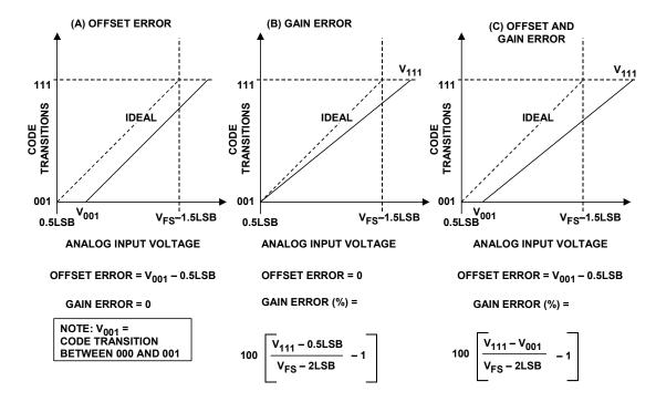
Figure 5.29: Measuring ADC Offset and Gain Error
