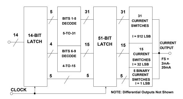
Figure 3.28: AD9775 TxDAC® 14-Bit CMOS DAC Core
