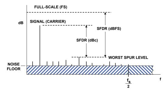
Figure 5.17: Measuring DAC Spurious Free Dynamic Range (SFDR)
