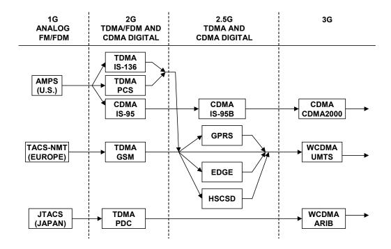
Figure 8.117: 1st Generation to 3rd Generation Wireless Evolution
