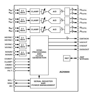
Figure 8.95: AD9888 100-/140-/170-/205-MSPS Analog Flat Panel Interface
