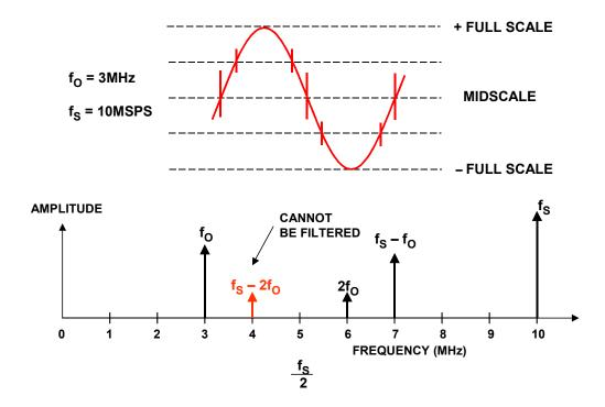
Figure 2.97: Effect of Code-Dependent Glitches on Spectral Output
