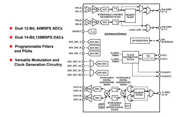
Figure 4.22: AD9860/AD9862 MxFE™ for Broadband Communications
