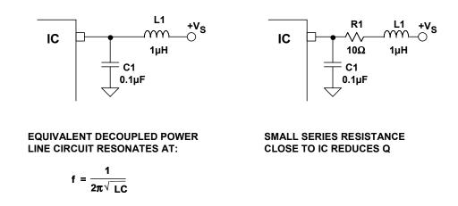
Figure 9.14: Resonant Circuit Formed by Power Line Decoupling
