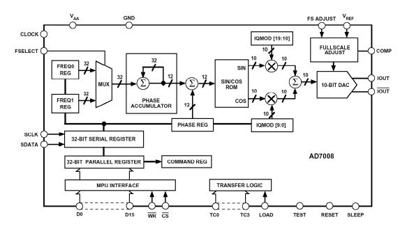
Figure 1.48: AD7008 10-Bit, 50-MSPS Complete CMOS DDS, 1993
