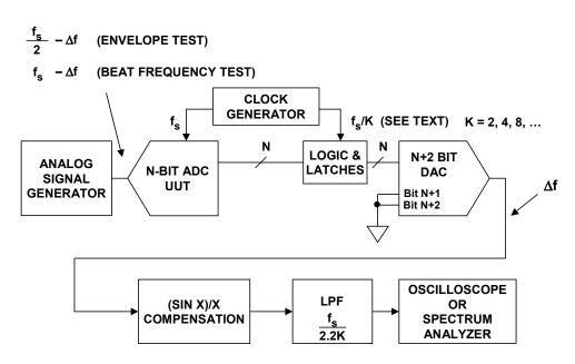
Figure 5.45: Envelope and Beat Frequency Test Setup
