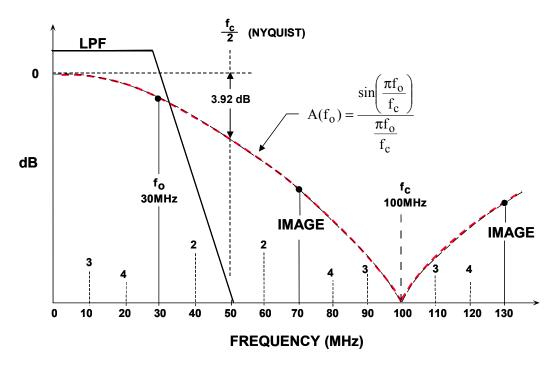
Figure 8.163: Aliasing in a DDS System Clocked at 100 MSPS with a 30-MHz Output
