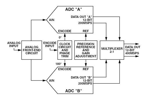
Figure 8.151: Two-Converter Time-Interleaved 12-Bit 400-MSPS ADC
