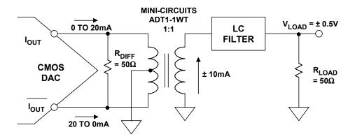
Figure 6.69: Differential Transformer Coupling
