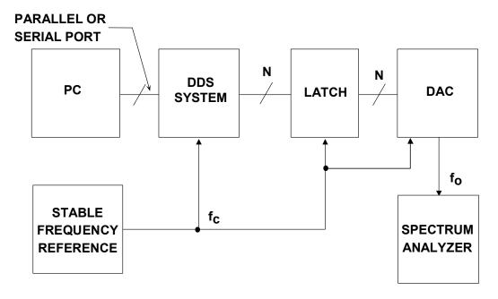
Figure 2.99: Test Setup for Measuring DAC SFDR
