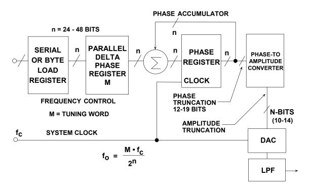
Figure 8.160: A Flexible DDS System
