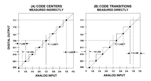
Figure 5.26: Measuring ADC Code Transistions to Determine Code Centers
