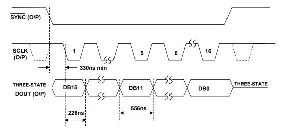
Figure 6.54: AD7853L Serial ADC Output Timing +3-V Supply, SCLK = 1.8 MHz
