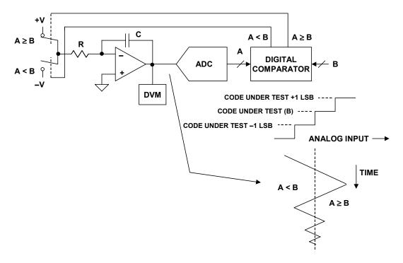
Figure 5.34: Integrating Servo-Loop ADC Tester
