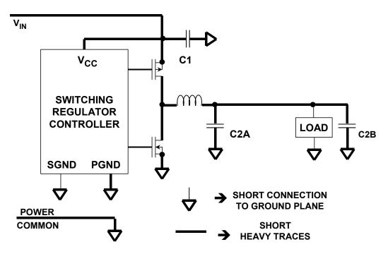
**Figure 9.66:** Grounding and Signal Routing Techniques for Switching Regulators Method 2
