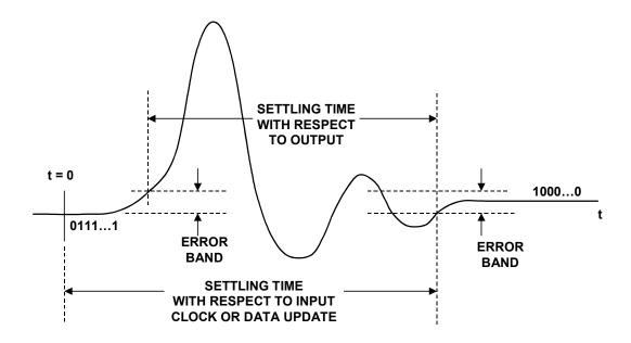
Figure 5.13: DAC Mid-Scale Settling Time Measurement
