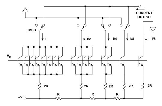
**Figure 3.21:** Binary-Weighted 4-Bit DAC: R/2R Ladder Network Current Setting Resistors
