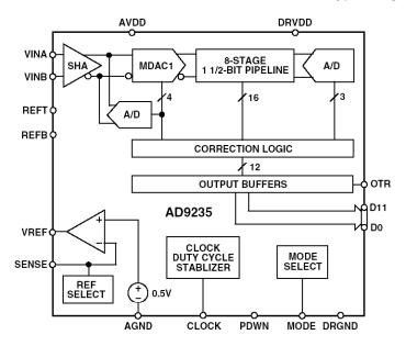
Figure 3.86: AD9235 12-Bit, 65-MSPS CMOC ADC, 2001
