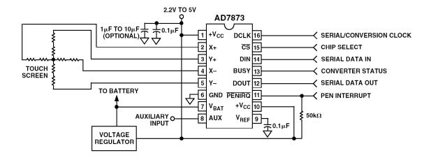
Figure 8.108: AD7873 Touchscreen Digitizer Application Circuit
