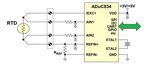
Figure 8.190: RTD Interfacing Using a MicroConverter
