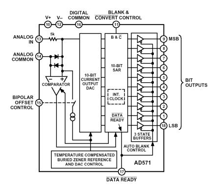
Figure 1.33: AD571 Complete 10-Bit, 25-µs IC ADC, 1978
