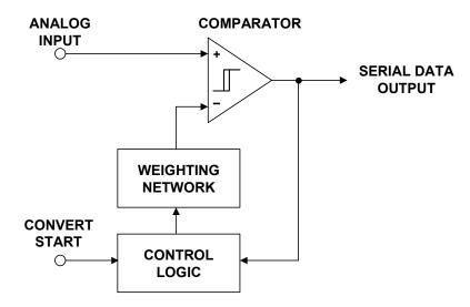
Figure 1.23: Basic Successive Approximation ADC (Feedback Subtraction ADC)
