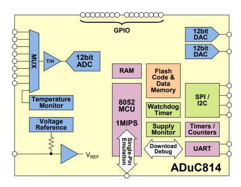
Figure 8.180: ADuC814 Reduced Pin-Count / Low Cost SAR MicroConverter®
