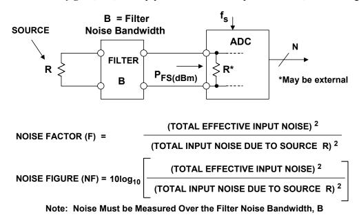
Figure 2.67: Noise Figure for ADCs: Use with Caution!
