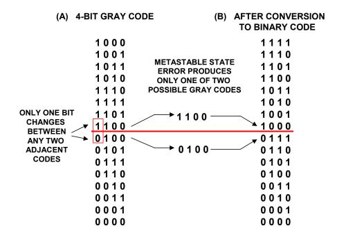
Figure 3.54: Gray Code Decoding Reduces
