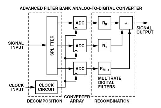
Figure 8.155: AFB Basic Block Diagram
