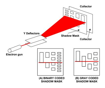
Figure 3.50: The Electron Beam Coder from Bell Labs (1948)
