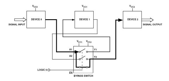
Figure 9.169: ADG3233 Bypass Switch in Bypass Mode
