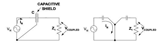
Figure 9.49: An Operational Model of a Faraday Shield
