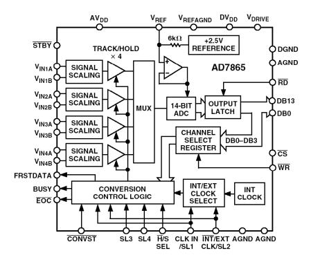
Figure 8.44: AD7865 4-Channel Simultaneous Sampling 14-Bit SAR ADC
