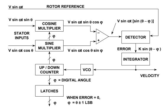
Figure 3.118: Resolver-to-Digital Converter (RDC)
