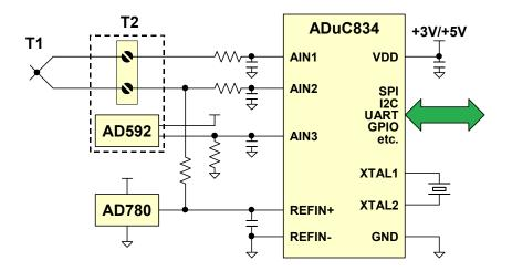
Figure 8.189: Thermocouple Interfacing Using a MicroConverter
