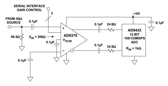
Figure 6.44: AD8370 Variable Gain Amplifier as a Low Distortion ADC Driver
