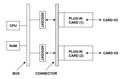
Figure 9.171: Using the ADG3247 in a Hot-Plug Application
