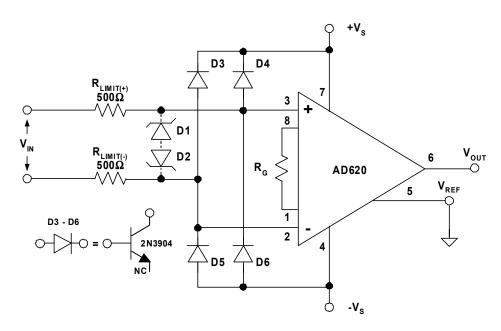
**Figure 9.85:** A Generalized Diode Protection Circuit for the AD620 and Other In-Amps Uses D3-D6 for CM Clamping and Series Resistors R<sub>LIMIT</sub> for Protection
