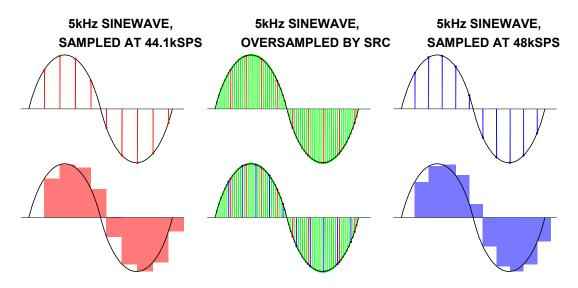
Figure 8.76: Conversion of a 5-kHz Sinewave from 44.1-kSPS to 48-kSPS Sample Rate
