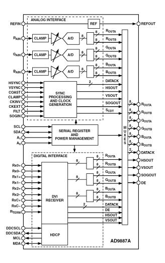
Figure 8.96: AD9887A Dual Flat Panel Interface
