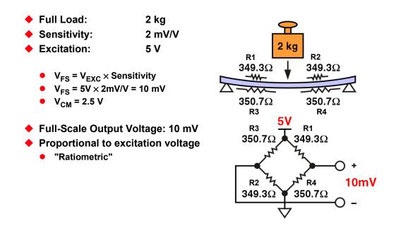
Figure 8.10: Determining Fullscale Output of Load Cell with 5-V Excitation
