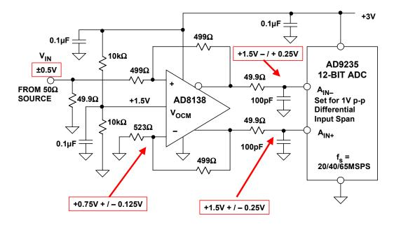
Figure 6.37: AD8138 Driving AD9235 12-Bit, 20-/40-/65-MSPS ADC
