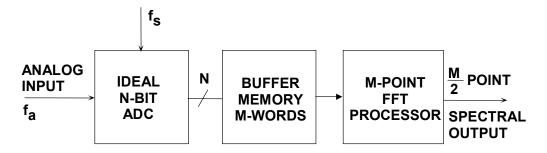
Figure 2.42: Dynamic Performance Analysis of an Ideal N-bit ADC
