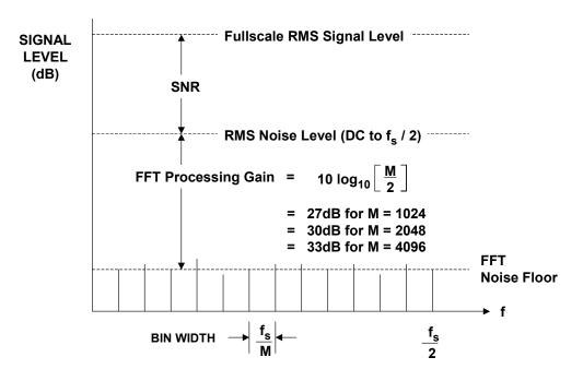
Figure 5.54: FFT Output Shows Effects of Processing Gain
