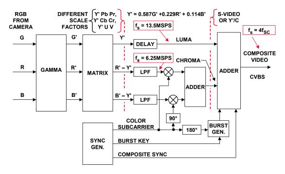
Figure 8.82: Model for Generating the Composite Video Signal from RGB Components
