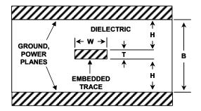
Figure 9.142: A Symmetric Stripline Transmission Line With Defined Impedance is Formed by a PCB Trace of Appropriate Geometry Embedded Between Equally Spaced Ground and/or Power Planes
