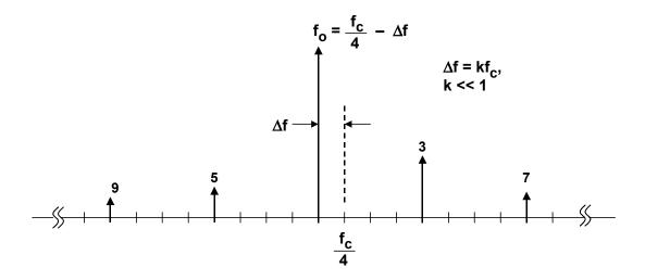
**Figure 5.24:** Location of Odd Harmonics for  $f_0 = f_0/4 - \Delta f$
