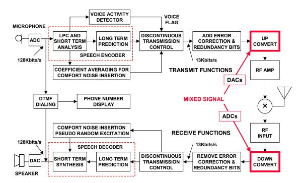
Figure 8.145: GSM Handset Block Diagram
