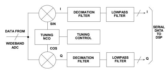
Figure 8.116: Receive Signal Processing (RSP) in Wideband Receiver (Simplified)
