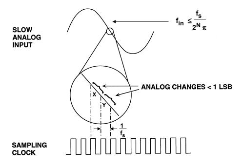
Figure 2.90: ADC Analog Signal for Low Frequency BER Test
