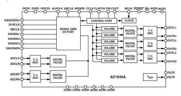
Figure 8.72: AD1839A, 2 ADC, 6 DAC, 96-kSPS 24-Bit  $\Sigma$ - $\Delta$  Codecs
