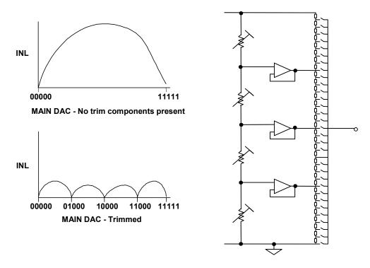
Figure 3.6: Trimming the INL of a String DAC (If Required)
