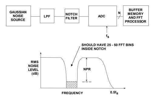
Figure 5.74: Noise Power Ratio (NPR) Test Setup
