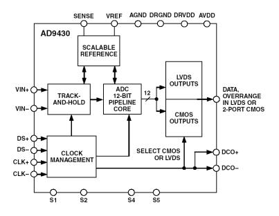
Figure 3.87: AD9430 12-Bit, 170-/210-MSPS ADC, 2002
