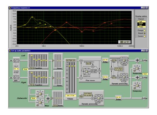
Figure 8.71: AD1953 SigmaDSP™ 3-Channel, 26-Bit Signal Processing DAC
