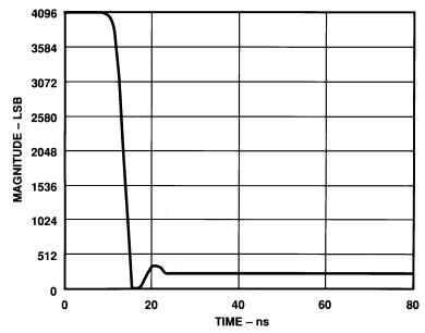
Figure 2.83: ADC Transient Response (Settling Time)
