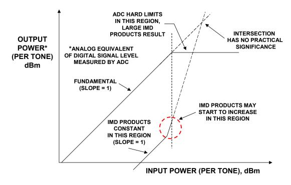
Figure 2.59: Intercept Points for Data Converters Have No Practical Significance
