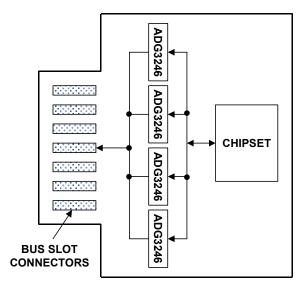
Figure 9.170: Hot Swapping with the ADG3246 Bus Switch
