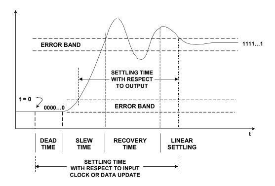
Figure 5.12: DAC Full-Scale Settling Time Measurement
