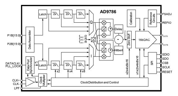
Figure 8.140: AD9786 16-Bit, 160-MSPS TxDAC+® with 2×/4×/8× Interpolation and Signal Processing
