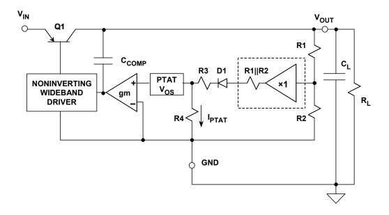
**Figure 9.56:** The ADP33xx anyCAP<sup>®</sup> LDO Architecture Has Both DC and AC Performance Advantages
