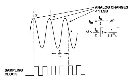
Figure 2.91: ADC Analog Input for High Frequency BER Test
