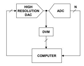
Figure 5.35: Generalized Computer Controlled Servo-Loop ADC Tester
