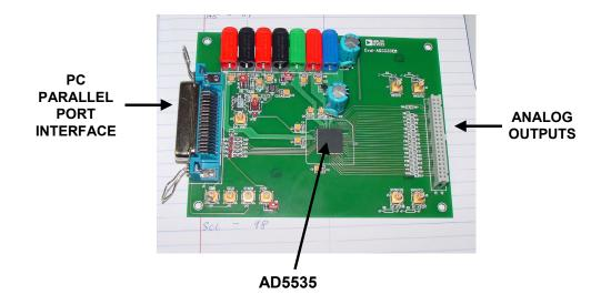
Figure 9.184: AD5535 32-Channel, 14-Bit, 200V Output DAC Evaluation Board
