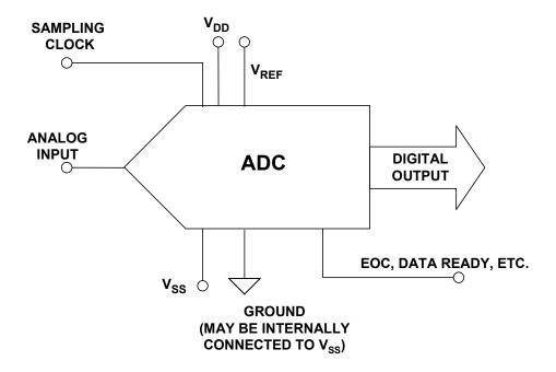
Figure 3.43: Basic ADC with External Reference
