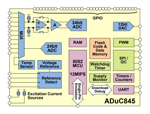
**Figure 8.184:** ADuC845/ADuC847/ADuC848 High Channel-Count, Fast Core Σ-Δ Based MicroConverter
