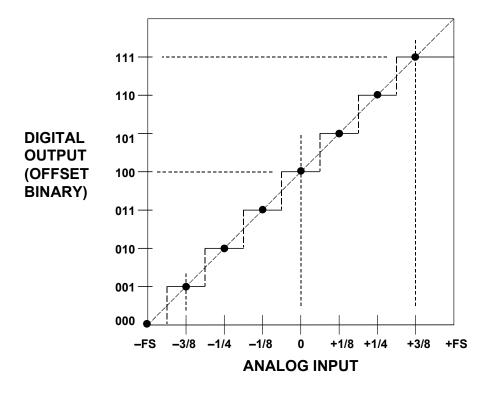
Figure 2.11: Transfer Function for Ideal Bipolar 3-bit ADC
