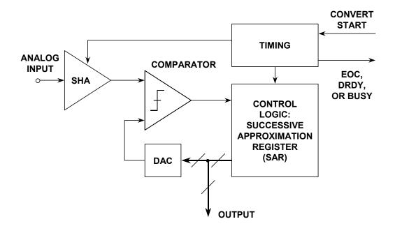
Figure 3.56: Basic Successive Approximation ADC (Feedback Subtraction ADC)
