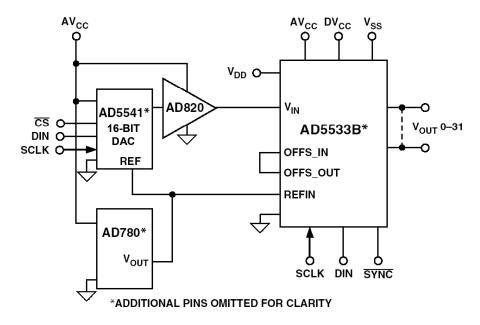
Figure 8.53: AD5533B Infinite Sample-and-Hold Typical Application Circuit
