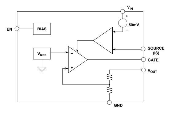
Figure 7.49: Functional Block Diagram of anyCAP Series
