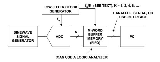
Figure 5.62: FFT Test Setup
