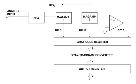
Figure 3.94: 3-bit Folding ADC Block Diagram
