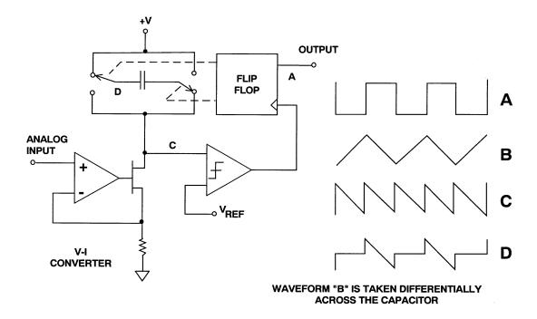
Figure 3.108: A Current-Steering VFC
