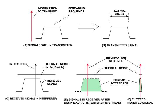
Figure 8.126: Signals Within a CDMA System
