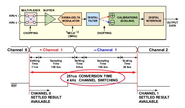
Figure 8.42: AD7739 Timing Showing Channel Switching
