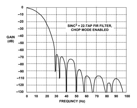
Figure 8.5: AD7730 Digital Filter Frequency Response
