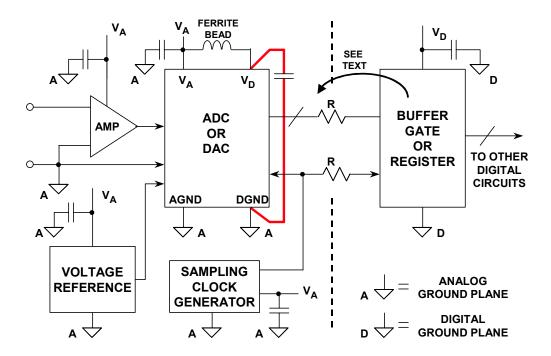
Figure 9.27: Grounding and Decoupling Points
