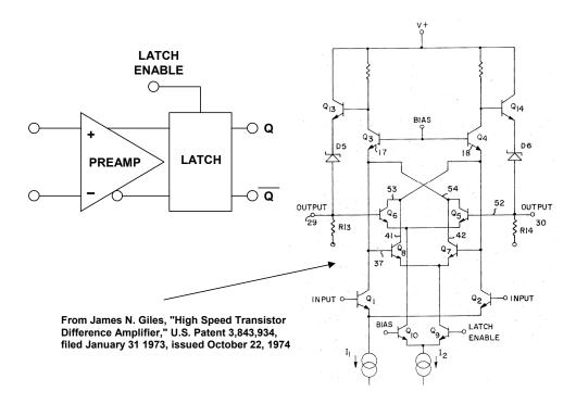
Figure 3.46: The AM685 ECL Comparator (1972)
