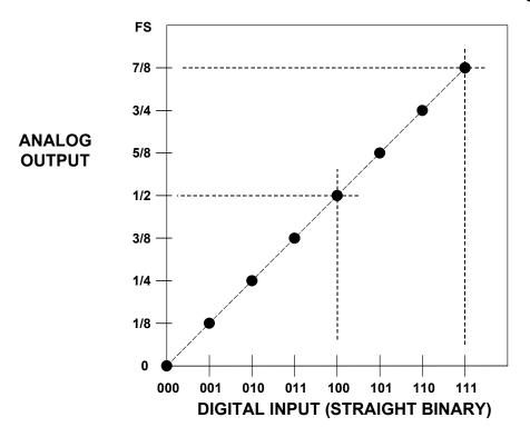
Figure 2.4: Transfer Function for Ideal Unipolar 3-bit DAC
