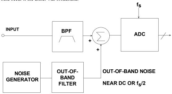
Figure 8.131: Injecting Out-of-Band Dither to Improve ADC SFDR
