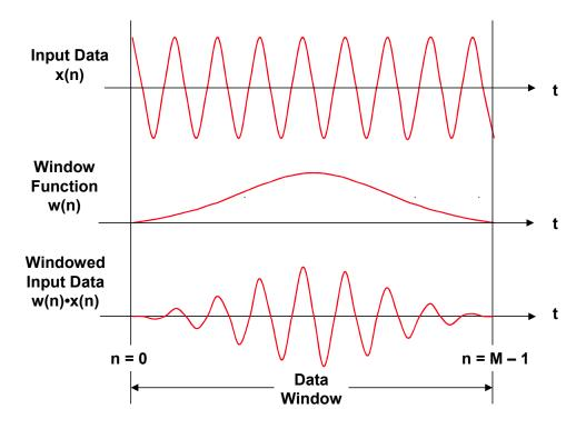
Figure 5.57: Windowing to Reduce Spectral Leakage
