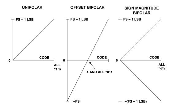
Figure 2.16: Unipolar and Bipolar Converters
