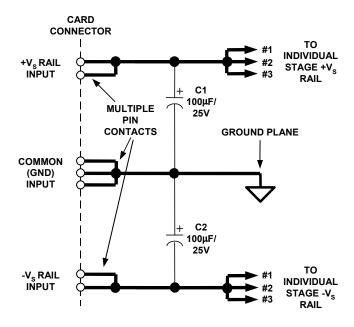
Figure 9.72: Dual-Supply Low Frequency Rail Bypass/Distribution Filter
