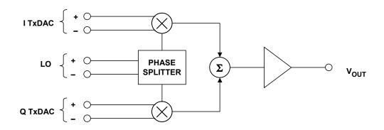
Figure 8.144: AD8349 800-MHz to 2.7-GHz Quadrature Modulator
