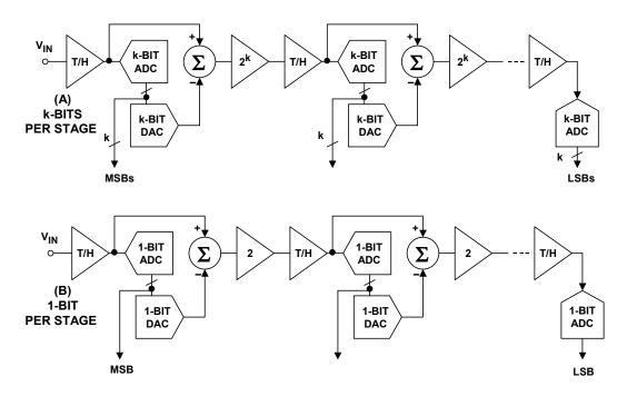
Figure 3.76: Basic Pipelined ADC with Identical Stages
