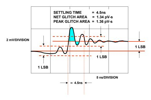
Figure 2.96: DAC Mid-scale Glitch Shows 1.34pV-s Net Impulse Area and Settling Time of 4.5ns
