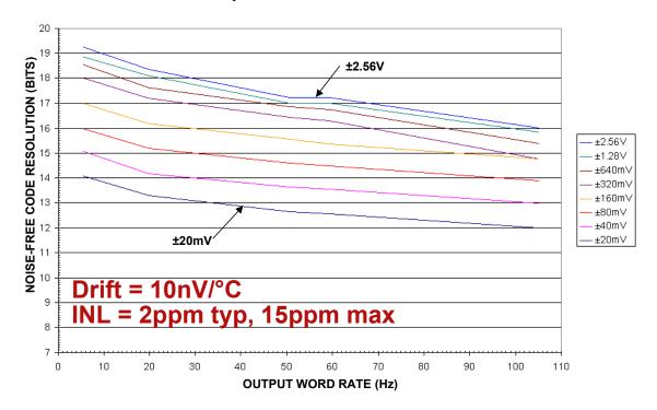
**Figure 8.185:** Σ-Δ ADC Performance – Normal Mode
