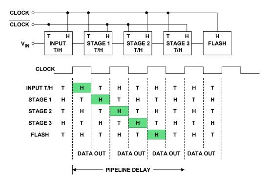
Figure 3.74: Clock Issues in Pipelined ADCs
