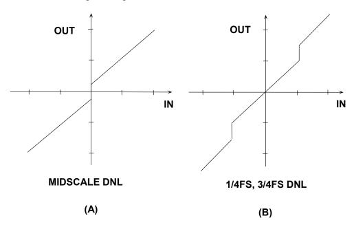
Figure 2.49: Typical ADC/ DAC DNL Errors (Exaggerated)
