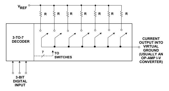
Figure 3.7: The Simplest Current-Output Thermometer (Fully-Decoded) DAC
