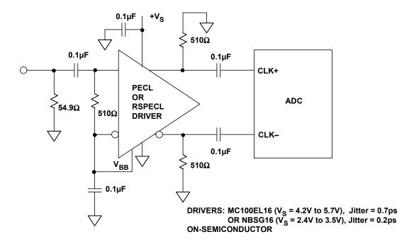
Figure 6.94: Low Jitter Single-Ended to Differential Clock Drivers
