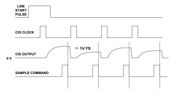
Figure 8.103: Contact Image Sensor (CIS) Waveforms
