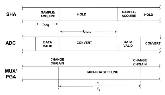
Figure 8.36: Typical Timing Diagram for Multiplexed Data Acquisition System Using a SHA
