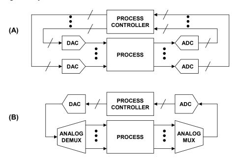
Figure 8.32: Two Approaches to a Multichannel Data Acquisition System
