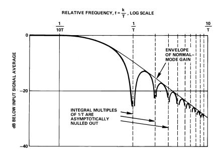
Figure 3.115: Frequency Response of Integrating ADC
