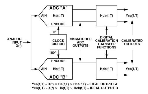
Figure 8.154: Example of Digital Post-Processing Architecture
