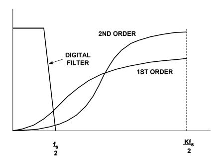
Figure 3.129: Sigma-Delta Modulators Shape Quantization Noise
