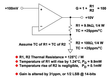
**Figure 9.5:** Uneven Power Dissipation Between Resistors With Identical TCs Can Also Introduce Temperature-Related Gain Errors
