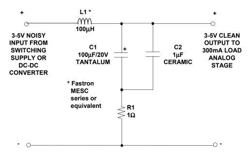
Figure 9.71: A Card-Entry Filter is Useful for Low-Medium Frequency Power
