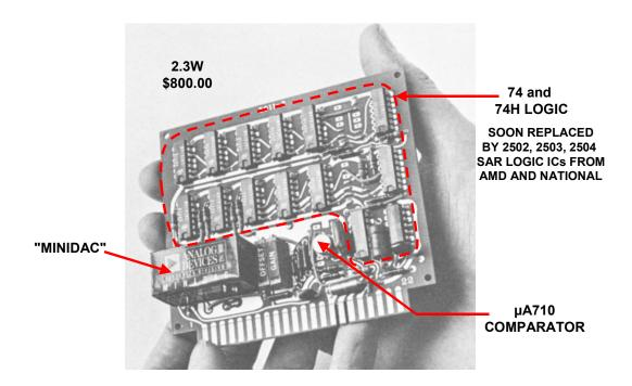
**Figure 1.19:** ADC-12U 12-Bit, 10-μs SAR ADC from Pastoriza Division of Analog Devices, 1969
