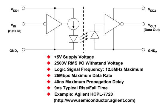
Figure 9.93: Digital Isolation Using LED / Photodiode Optocouplers
