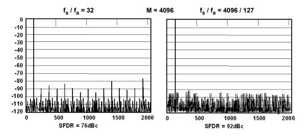
Figure 2.43: Effect of Ratio of Sampling Clock to Input Frequency on SFDR for Ideal 12-bit ADC
