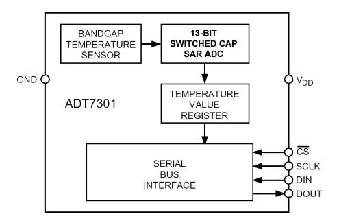
**Figure 8.23:** ADT7301 13-Bit, ±0.5°C Accurate, Micropower Digital Temperature Sensor
