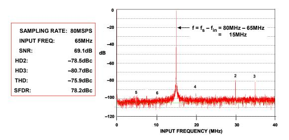
**Figure 6.42:** AD8351 Differential ADC Driver Performance with AD6645 ADC (G = 10 dB)
