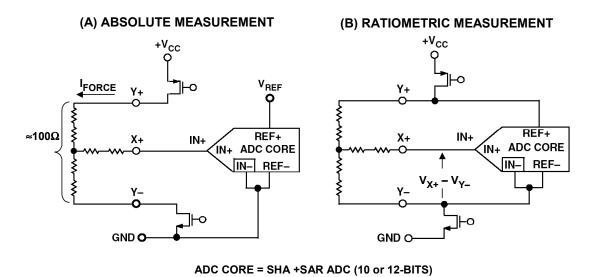
Figure 8.106: Absolute and Ratiometric Measurements of Touchscreen Voltages
