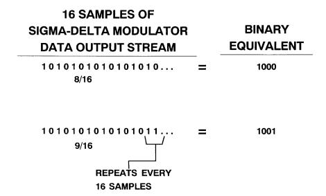
Figure 3.132: Repetitive Bit Pattern in Sigma-Delta Modulator Output
