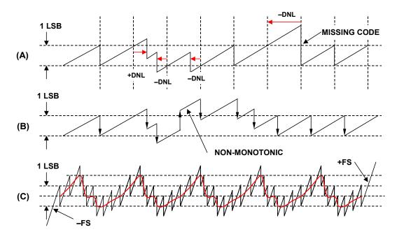
Figure 5.31: ADC Error Waveforms Using "Back-to-Back" Test Setup
