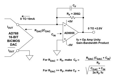
Figure 6.72: Single-Ended I/V Op Amp Interface for Precision 16-Bit AD768 DAC
