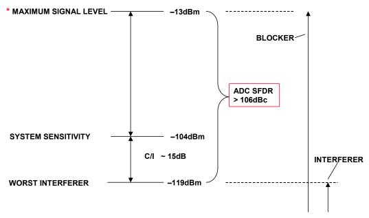
\* NOTE: MAXIMUM SIGNAL LEVEL FOR GSM 1800MHz/1900MHz AND PCS SPEC = -23dBm
