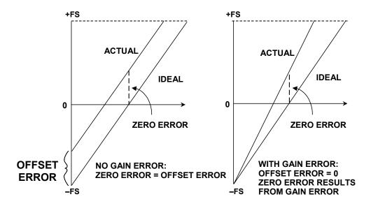
Figure 2.17: Bipolar Data Converter Offset and Gain Error
