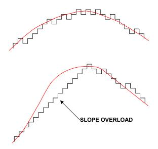
Figure 3.120: Quantization Using Delta Modulation
