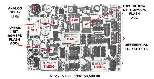
Figure 1.41: MOD-1020, 10-Bit, 20-MSPS Sampling ADC Introduced in 1979
