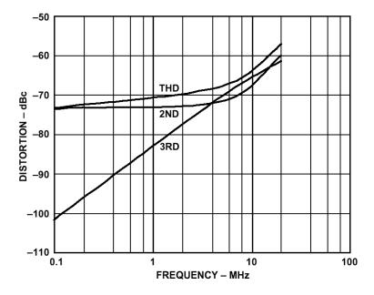
**Figure 6.14:** AD8057/AD8058 Op Amp Distortion Versus Frequency G = +1.  $R_1 = 150 \Omega$ .  $V_S = \pm 5 V$
