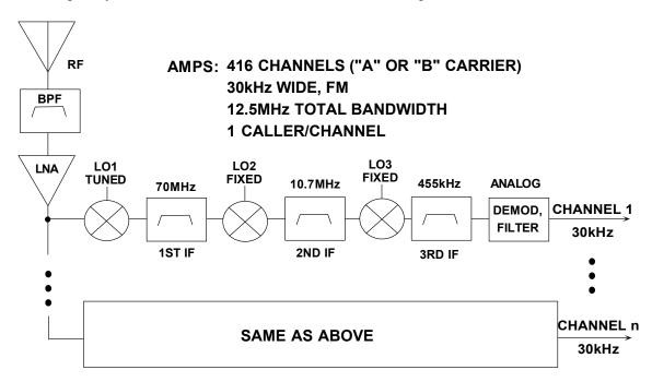
**Figure 8.110:** U.S. Advanced Mobile Phone Service (AMPS) Superheterodyne Analog Receiver
