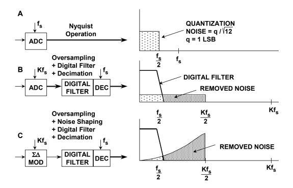
Figure 3.125: Oversampling, Digital Filtering, Noise Shaping, and Decimation
