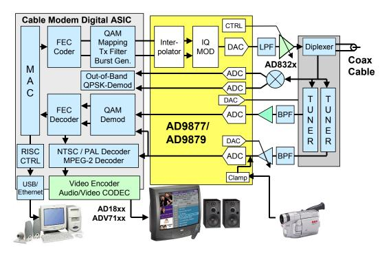
**Figure 4.18:** AD9877 / AD9879 Set-Top Box Mixed Signal Front End (MxFE™)
