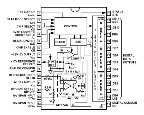
Figure 1.34: The Industry-Standard AD574 12-Bit, 35-μs IC ADC, 1978
