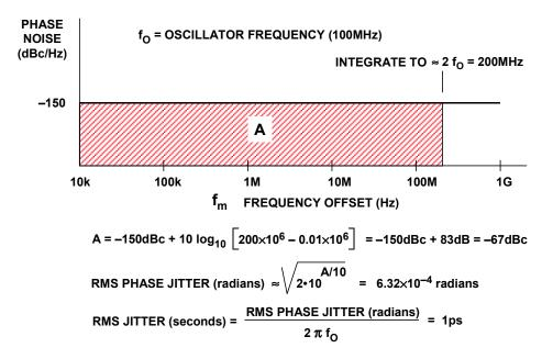
Figure 6.85: Sample Jitter Calculation Assuming Broadband Phase Noise
