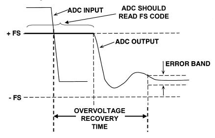
Figure 2.86: Overvoltage Recovery Time
