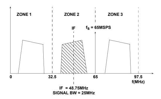
**Figure 8.128**: Sampling a 25-MHz BW Signal Using AD6645: IF Frequency = 48.75 MHz,  $f_s = 65 \text{ MSPS}$
