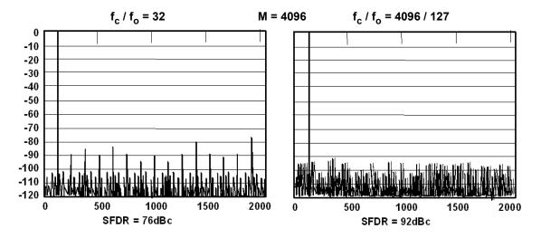
**Figure 5.20:** Effect of Ratio of Sampling Clock f<sub>c</sub> to Output Frequency f<sub>o</sub> on SFDR for Ideal 12-bit DAC
