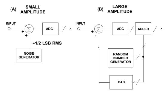
Figure 8.130: Using Dither to Randomize ADC Transfer Function
