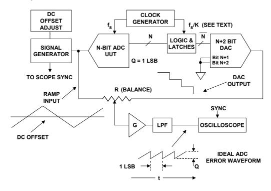
Figure 5.30: ADC/DAC Back-to-Back Static Testing
