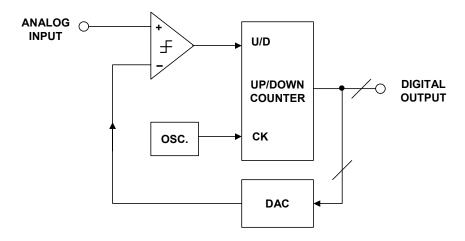
Figure 3.106: Tracking ADC
