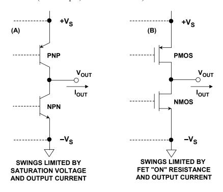
Figure 6.9: "Almost" Rail-To-Rail Output Stages
