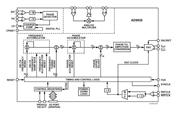
Figure 8.169: AD9858 1-GSPS DDS with Phase Detector and Analog Multiplier
