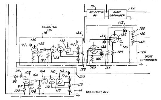
Extracted from: John C. Schelleng, "Code Modulation Communication System," U.S. Patent 2,453,461, Filed June 19, 1946, Issued November 9, 1948
