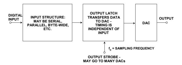
Figure 6.61: Double-Buffered DAC Permits Complex Input Structures and Simultaneous Update
