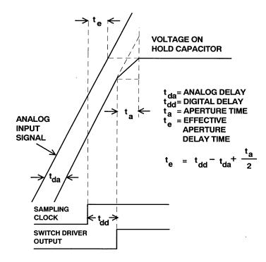
Figure 7.104: SHA Waveforms
