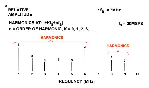
Figure 2.50: Location of Distortion Products: Input Signal = 7 MHz, Sampling Rate = 20 MSPS
