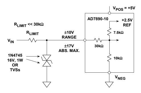
**Figure 9.89:** Input Protection for Single-Supply ADCs With Thin Film Resistor Input Attenuators
