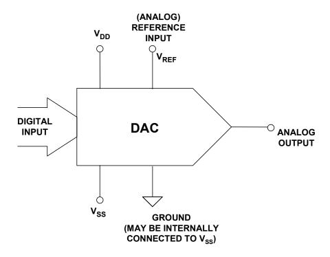
Figure 3.1: Basic DAC with External Reference
