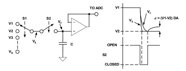
Figure 9.3: Dielectric Absorption Induces Errors in SHA Applications
