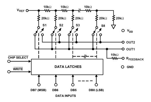
Figure 1.31: AD7524 8-Bit Buffered μP Compatible DAC, 1978
