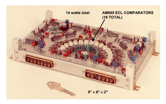
Figure 3.52: MOD-4100 4-Bit, 100-MSPS Flash Converter, Computer Labs, 1975
