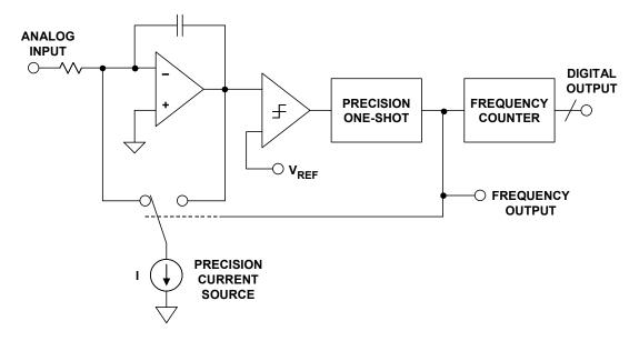
Figure 3.109: Charge Balance Voltage-to-Frequency Converter (VFC)
