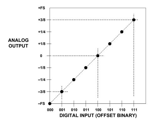
Figure 2.10: Transfer Function for Ideal Bipolar 3-bit DAC
