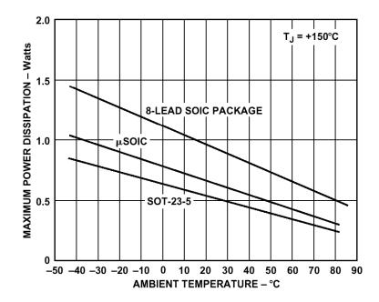
**Figure 9.115:** Comparative Thermal Performance for Several AD8057/58 Op Amp Package Options
