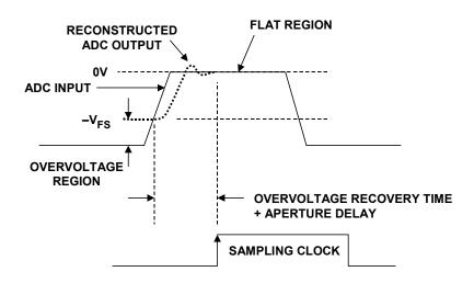
Figure 5.82: Overvoltage Recovery Test Waveform from Flat Pulse Generator
