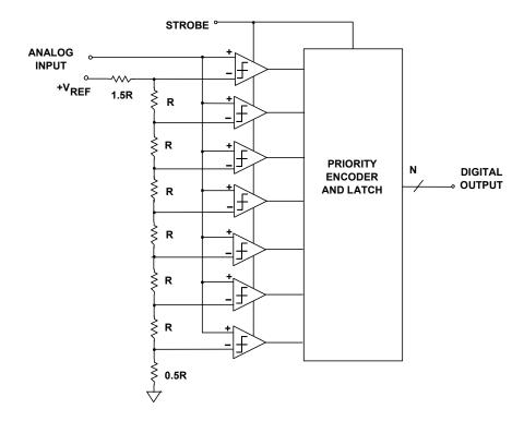
Figure 3.48: 3-bit All-Parallel (Flash) Converter
