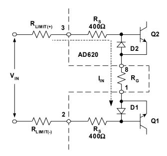
**Figure 9.84:** The AD620 In-Amp Input Internally Uses D1-D2 and Series Resistors R<sub>S</sub> for Protection (Additional Protection Can Be Added Externally)
