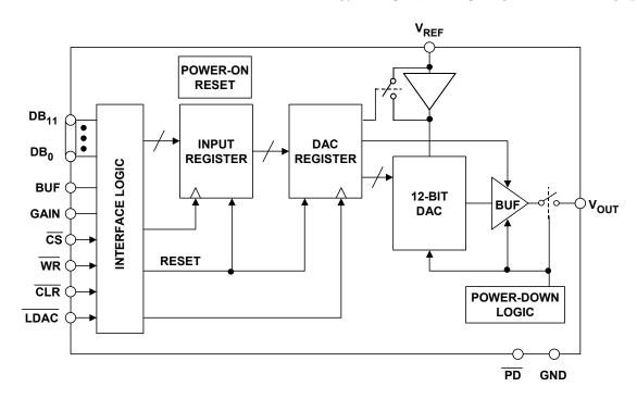
Figure 6.64: AD5340 12-Bit, 100-kSPS Parallel Input DAC
