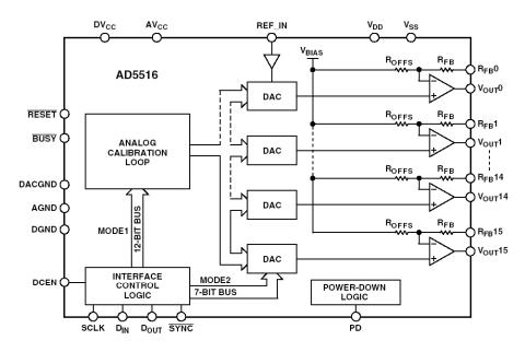
Figure 8.49: AD5516 16-Channel 12-Bit Voltage Output DAC
