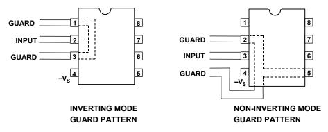
Figure 9.45: PCB Guard Patterns for Inverting and Non-Inverting Mode Op Amps Using 8 Pin SOIC (R) Package
