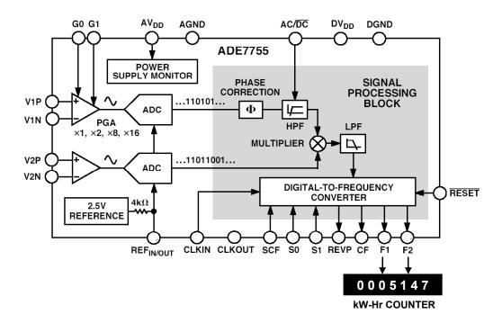
Figure 8.30: ADE7755 Energy Metering IC with Pulse Output
