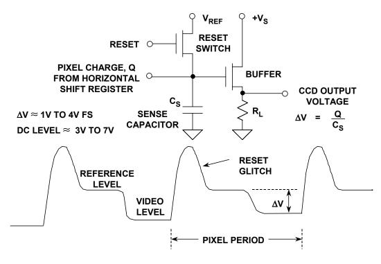
Figure 8.100: Output Stage and Waveforms
