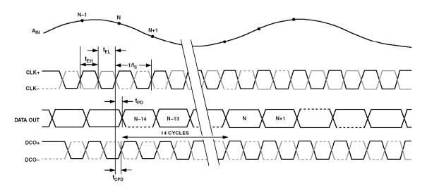
Figure 6.57: AD9430 LVDS Output Data Timing
