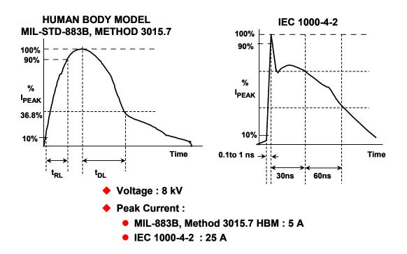
Figure 9.106: ESD Test Waveforms
