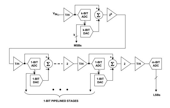
Figure 3.77: Multibit and 1-Bit Pipelined Core Combined
