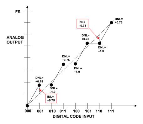
Figure 5.9: DNL Specification of < ±1 LSB Does Not Guarantee INL < ±0.5 LSB
