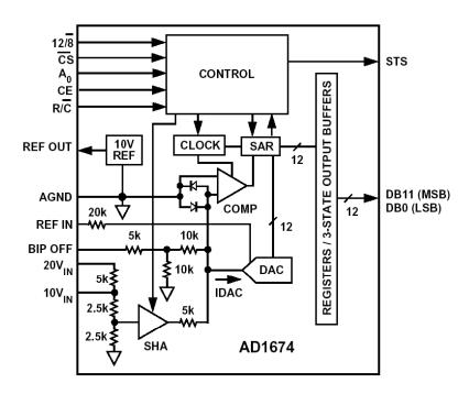
**Figure 1.50:** AD1674, 12-Bit, 100-kSPS Sampling ADC (AD574 Pin-Compatible), 1990
