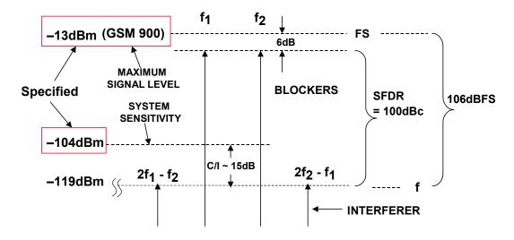
NOTE: MAXIMUM SIGNAL LEVEL FOR GSM 1800/1900 SPEC = -23dBm
