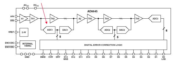
Figure 8.132: AD6645 Subranging Point DNL Errors (Exaggerated)
