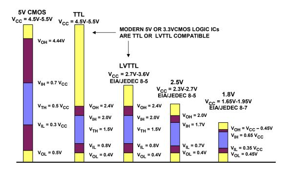
Figure 9.157: Standard Logic Levels
