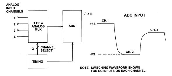
Figure 2.84: Settling Time is Critical in Multiplexed Applications
