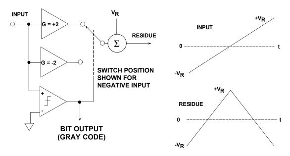
Figure 3.93: Folding Stage Functional Equivalent Circuit
