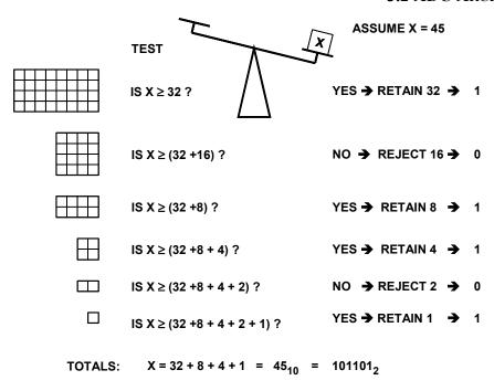
Figure 3.59: Successive Approximation ADC Algorithm
