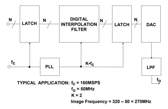
Figure 2.104: Oversampling Interpolating TxDAC® Simplified Block Diagram
