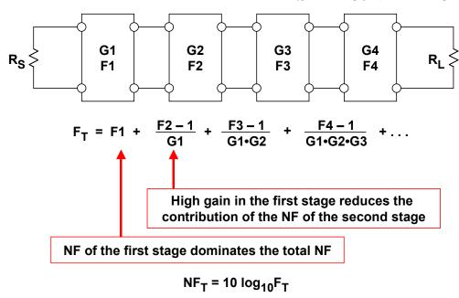
Figure 2.74: Cascaded Noise Figure Using the Friis Equation
