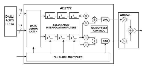
Figure 4.19: AD9777 TxDAC and AD8346 Quadrature Modulator
