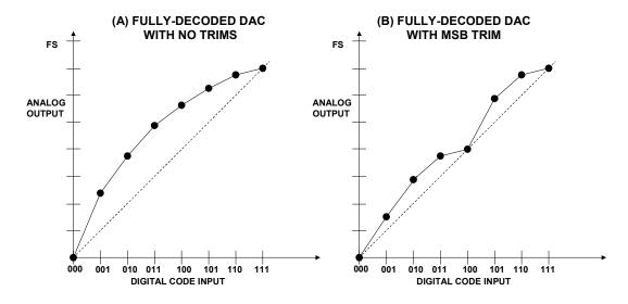
Figure 5.10: INL of Fully-Decoded 3-Bit DACs (String DACs)
