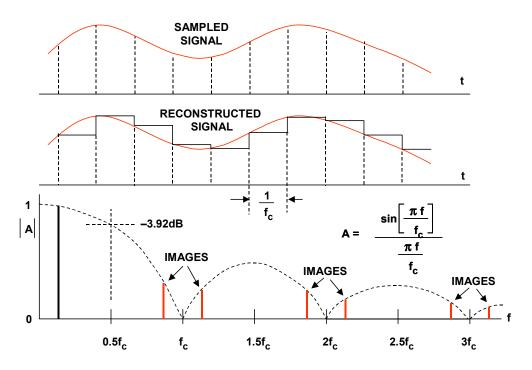
Figure 2.102: DAC sin x/x Roll Off (Amplitude Normalized)
