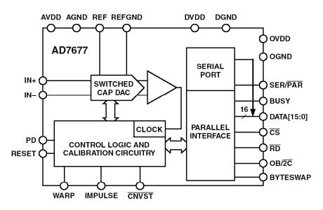
Figure 3.64: AD7677 16-Bit 1-MSPS Switched Capacitor PulSAR® ADC
