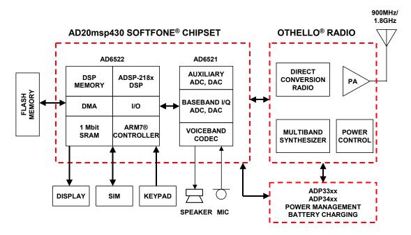
**Figure 8.146:** Othello<sup>®</sup> Radio and SoftFone<sup>®</sup> Chipsets Make Complete GSM/DCS Handset
