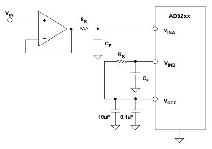
Figure 6.22: Optimizing a Single-Ended Switched Capacitor
