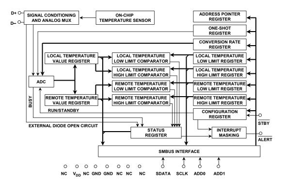
Figure 8.26: ADM1023 Simplified Block Diagram
