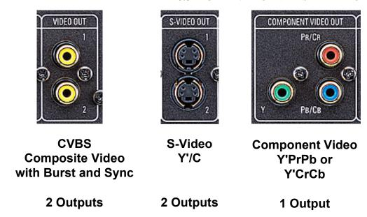
Figure 8.84: What the Analog Connectors Look Like on a High-End Receiver
