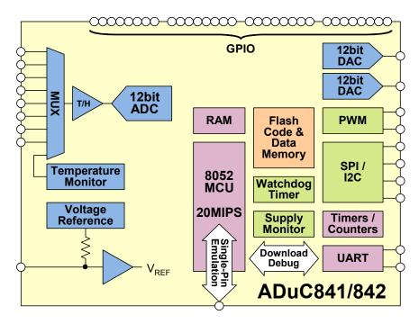
Figure 8.179: Standard SAR MicroConverter® Products ADuC812/831/832/841/842/843
