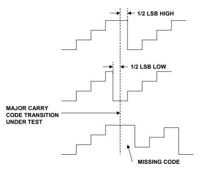
Figure 5.33: Crossplot Waveforms Showing ADC Static Errors
