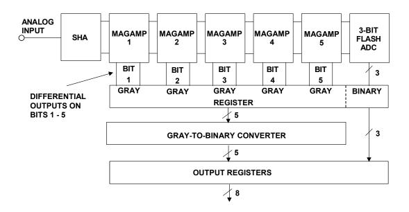
Figure 3.100: AD9054A 8-bit, 200-MSPS ADC Functional Diagram
