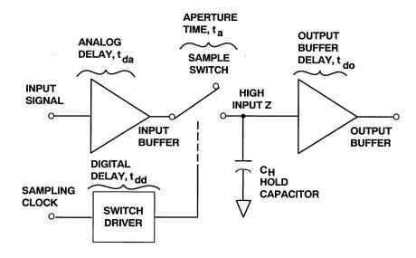
Figure 7.103: SHA Circuit Showing Internal Timing
