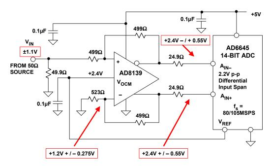
Figure 6.40: AD8139 Application as DC Coupled Driver for the AD6645 14-bit, 80-/105-MSPS ADC
