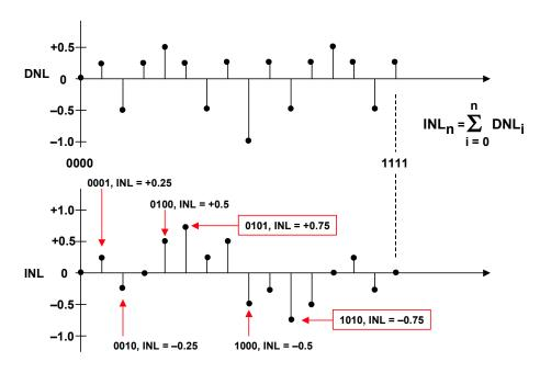
Figure 5.6: DNL and INL for 4-Bit DAC Where Superposition Holds
