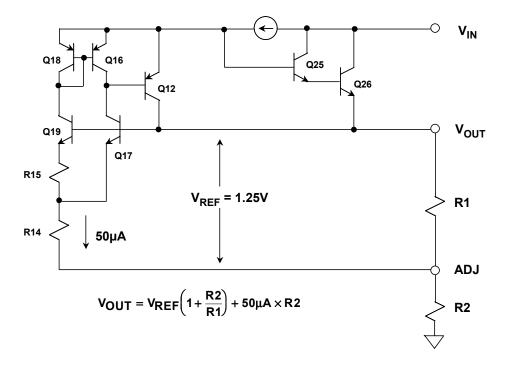
Figure 7.31: Simplified Schematic of LM317 Adjustable Three-terminal Regulator
