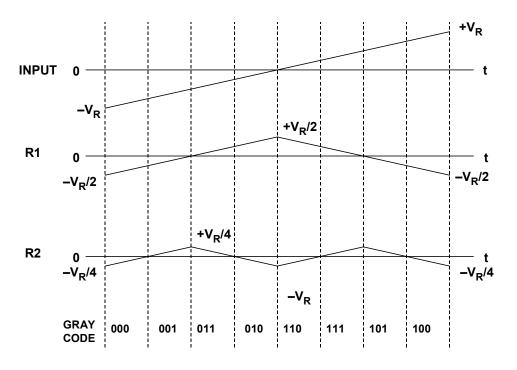
Figure 3.97: Single-Ended Waveforms in Chasek's Folding ADC
