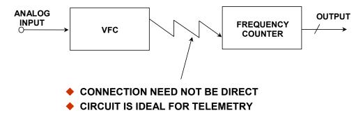
Figure 3.107: Voltage-to-Frequency Converter (VFC) and Frequency Counter
