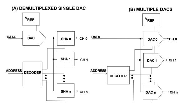
Figure 8.46: Options for Analog Data Distribution
