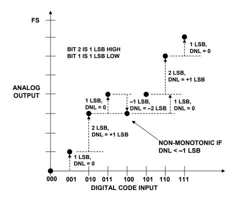
Figure 2.20: Details of DAC Differential Nonlinearity
