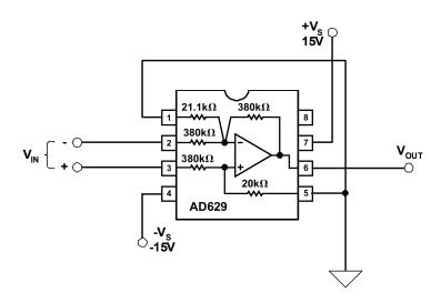
**Figure 9.79:** The AD629 High Voltage In-Amp IC Offers  $\pm$  500 V Input Overvoltage Protection, One-Component Simplicity, and Fail-Safe Power Off Operation
