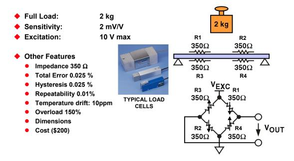
Figure 8.9: Load Cell Characteristics
