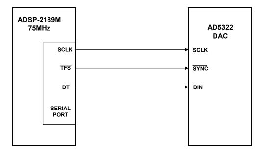
Figure 6.63: AD5322 DAC Serial Interface to ADSP-2189M
