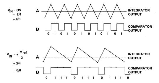
Figure 3.127: Sigma-Delta Modulator Waveforms
