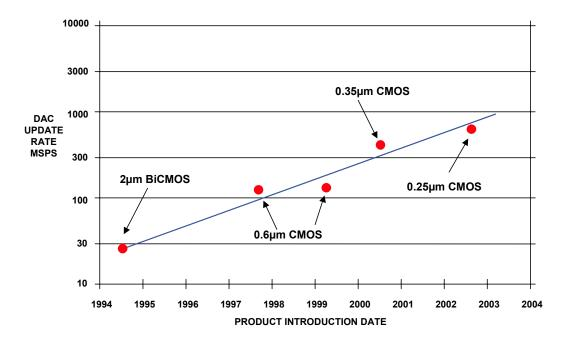
Figure 4.10: High-Speed DAC Update Rate Trend
