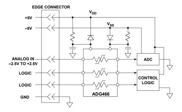
Figure 9.91: Overvoltage and Power Supply Sequencing Protection Using the ADG466
