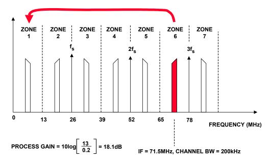
**Figure 8.113:** Narrowband GSM Receiver Bandpass Sampling of a 200-kHz Channel at 26 MSPS
