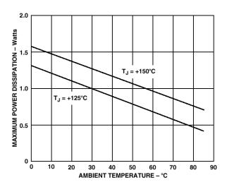
Figure 9.110: Thermal Rating Curves for AD8017AR Op Amp
