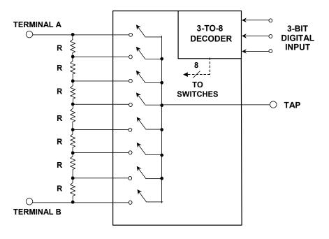
Figure 3.5: A Slight Modification to a String DAC Yields a "Digital Potentiometer"
