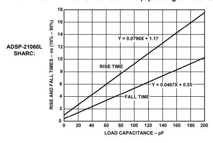
Figure 9.143: Typical DSP Output Rise Times and Fall Times
