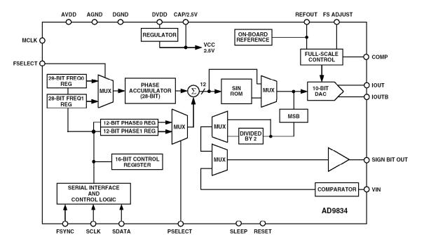
Figure 8.166: AD9834 Low Power (20mW), 50-MSPS DDS Synthesizer
