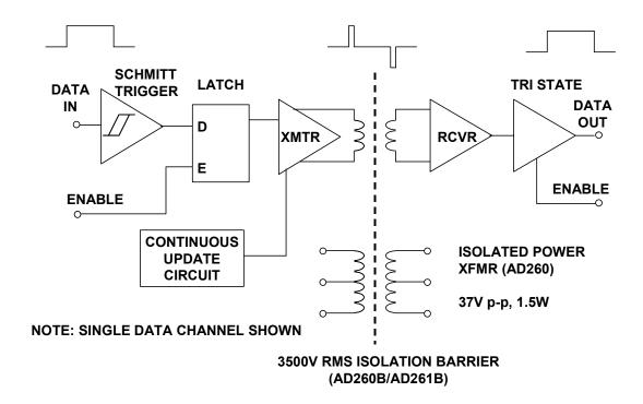
Figure 9.95: AD260/AD261 Digital Isolators
