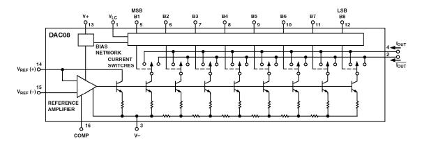
Figure 1.28: DAC08 8-Bit 85-ns IC DAC, 1975
