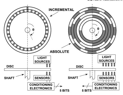
Figure 3.116: Incremental and Absolute Optical Encoders
