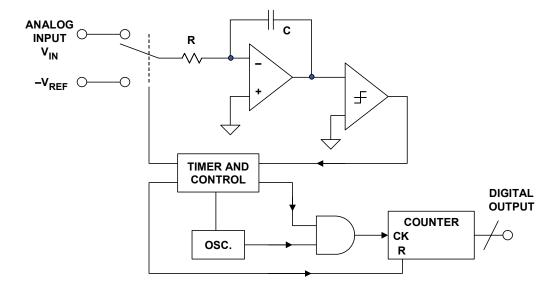
Figure 3.113: Dual slope ADC
