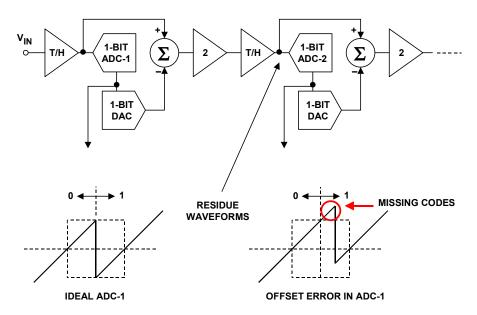
Figure 3.78: 1-Bit per Stage Pipelined ADC
