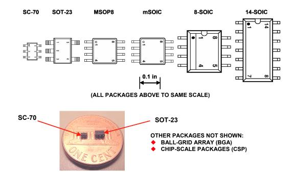
Figure 4.13: Examples of Modern Data Converter Packages
