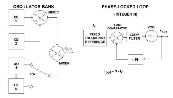
Figure 8.158: Frequency Synthesis Using Oscillators and Phase-locked Loops
