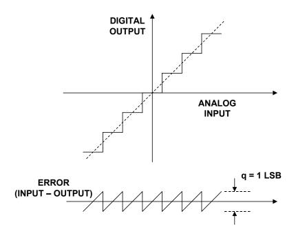
Figure 2.37: Ideal N-bit ADC Quantization Noise
