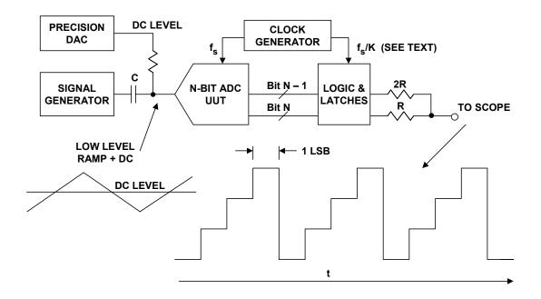
Figure 5.32: ADC Crossplot Test
