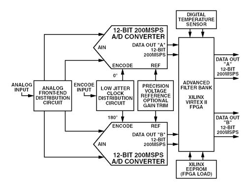
Figure 8.156: AD12400 12-Bit, 400MSPS ADC Block Diagram
