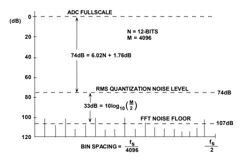
Figure 2.44: Noise Floor for an Ideal 12-bit ADC Using 4096-point FFT
