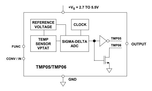
Figure 8.20: Digital Output Temperature Sensors: TMP05/06
