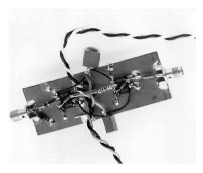
Figure 9.174: A "Deadbug" Analog Breadboard
