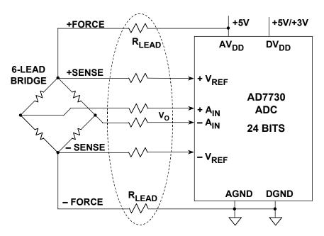
**Figure 8.7:** AD7730 Bridge Application Showing Ratiometric Operation and Kelvin Sensing
