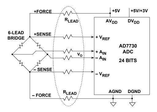
Figure 3.145: AD7730 Bridge Application (Simplified Schematic)
