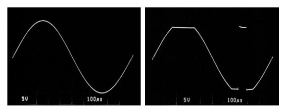
Figure 9.81: An Illustration of Input Overdriving Waveform (Left) and the Resulting Output Phase-Reversal (Right), Using a JFET Input Op Amp
