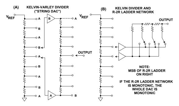
Figure 3.24: Segmented Voltage-Output DACs
