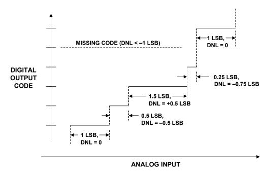
Figure 2.21: Details of ADC Differential Nonlinearity
