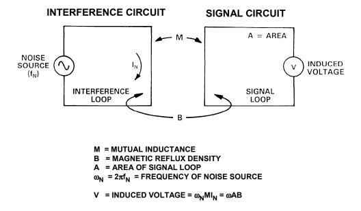
Figure 9.11: Basic Principles of Inductive Coupling
