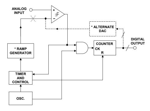
Figure 3.105: Ramp Run-Up ADC
