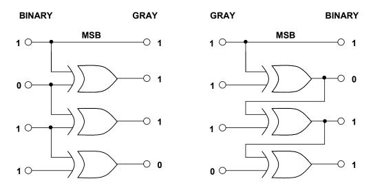
Figure 2.8: Binary-to-Gray and Gray-to-Binary Conversion Using the Exclusive-Or Logic Function
