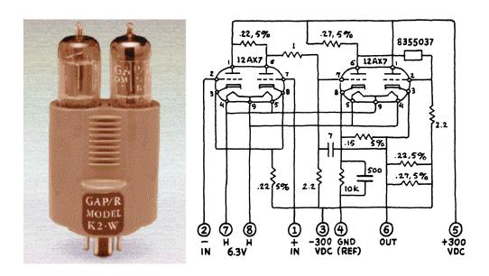
Figure 4.2: The K2-W Op Amp Introduced in 1953 (Courtesy of Dan Sheingold)
