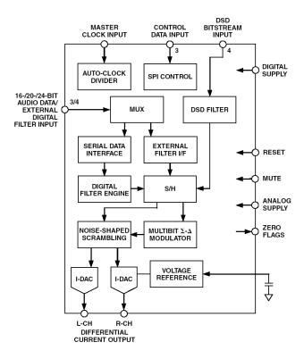
Figure 3.148: AD1955 Multibit Sigma-Delta Audio DAC
