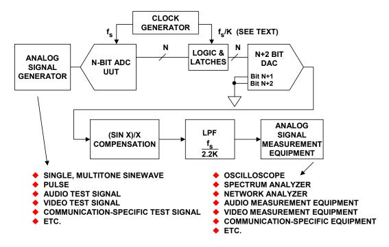
Figure 5.44: "Back-to-Back" Setup for ADC Dynamic Testing
