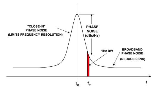
Figure 6.81: Oscillator Power Spectrum Due to Phase Noise
