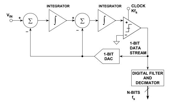
Figure 3.130: Second-Order Sigma-Delta ADC
