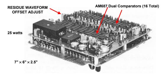
**Figure 3.68:** MOD-815, 8-Bit, 15 MSPS 4×4 Subranging ADC, 1976, Computer Labs, Inc.
