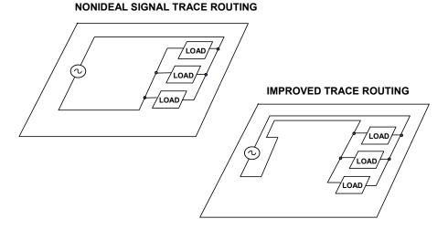
Figure 9.10: Nonideal and Improved Signal Trace Routing
