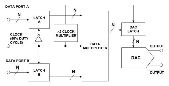
Figure 3.42: Alternate Loading (Ping-Pong) High Speed DAC
