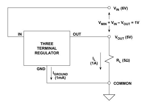
Figure 9.53: A Basic Three Terminal Regulator Hookup (Either Positive or Negative)
