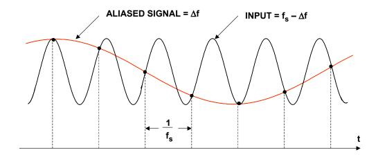
NOTE: INPUT IS SLIGHTLY LESS THAN f<sub>s</sub>
