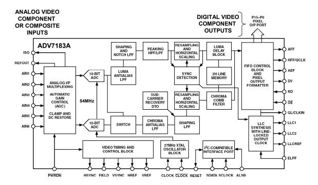
Figure 8.85: ADV7183A 10-Bit Video Decoder
