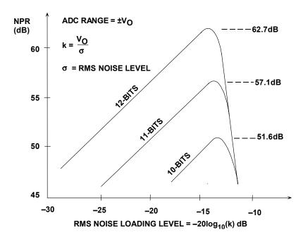
Figure 2.64: Theoretical NPR for 10, 11, 12-bit ADCs
