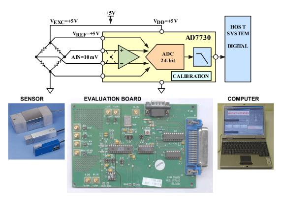
Figure 9.183: AD7730 Measurement ADC Evaluation System
