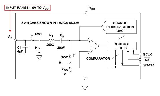
Figure 6.18: Input Circuit of AD7466 1.6-V to 3.6-V, 12-Bit, 200-kSPS SOT-23-6 ADC
