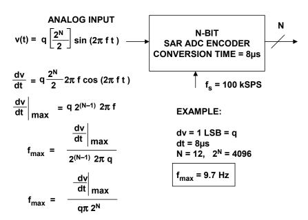
Figure 2.26: Input Frequency Limitations of Non-Sampling ADC (Encoder)
