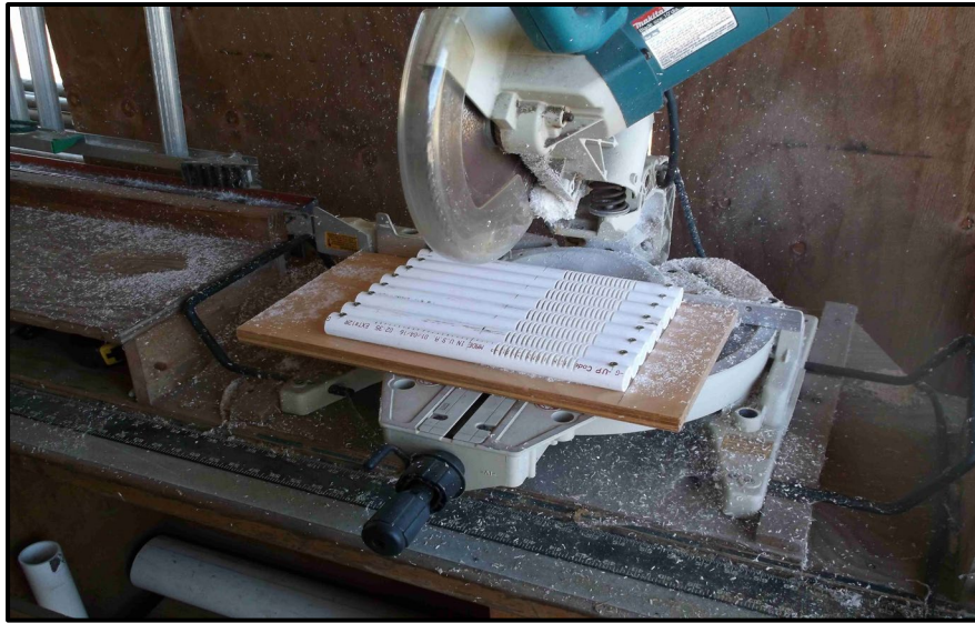
Figure 6.18 - Cutting the wire slots.
