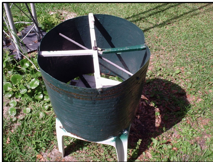
Figure 6.19 - Pat W5THT, foil wound lightweight inductor.
