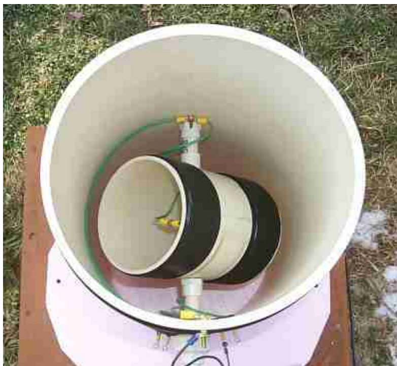
Figure 6.38B - Jay, W1VD, WD2XNS variometer.
