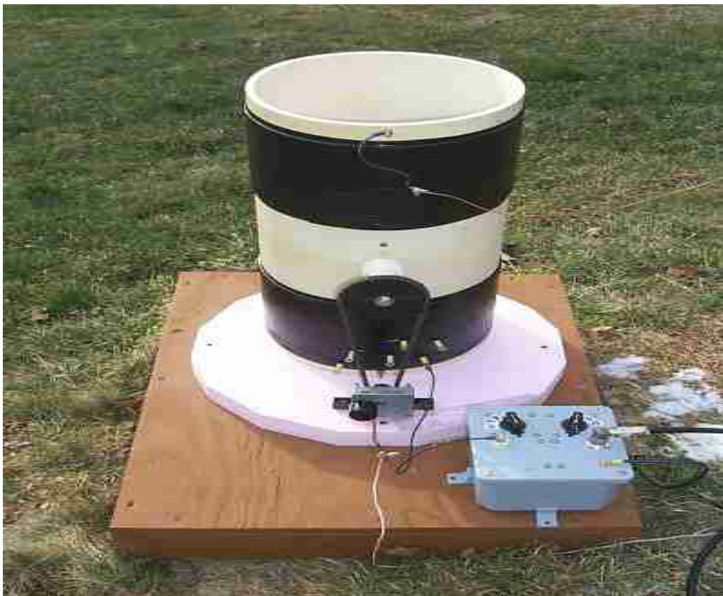
Figure 6.38A - Jay, W1VD, WD2XNS variometer.
