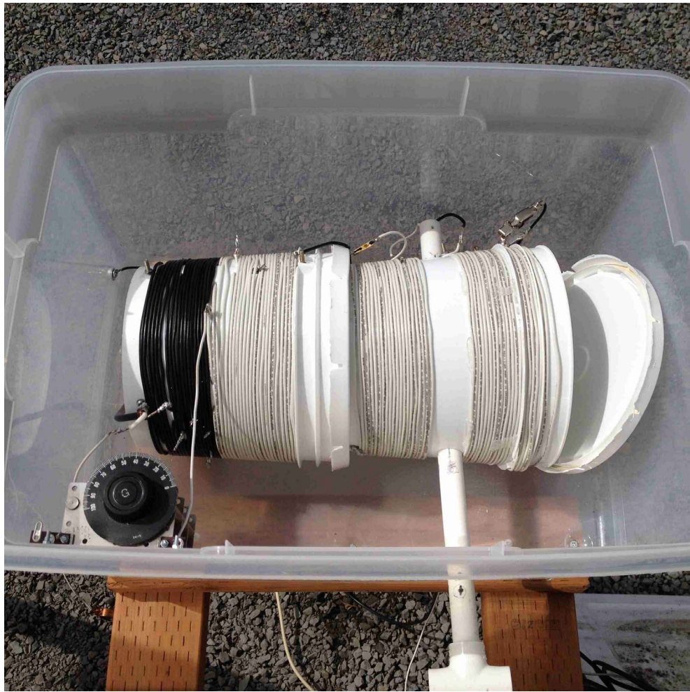
Figure 6.40A -Neil, W0YSE, variometer.
