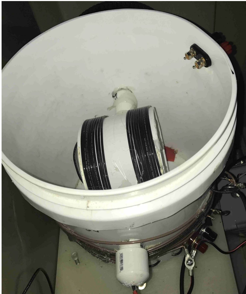
Figure 6.36 - Laurence, KL7L. Bucket variometer example.
